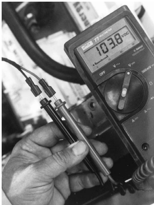
Above: A pair of insulated connectors make a convenient test point for measuring full battery voltage.
