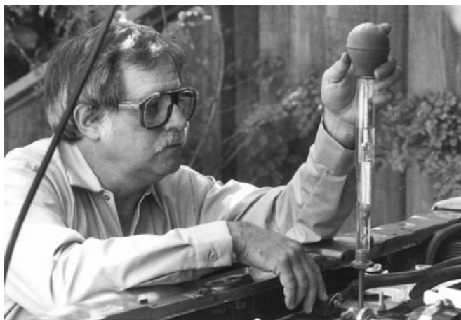
Above: Testing specific gravity with a hydrometer will pinpoint weak batteries.
