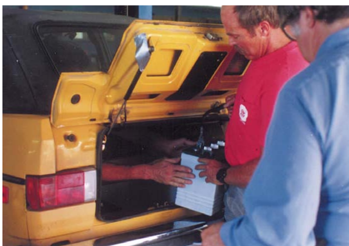
Top: Batteries are added to the front of the VW. Center and Bottom: The rear compartment is modified to also accept batteries.
