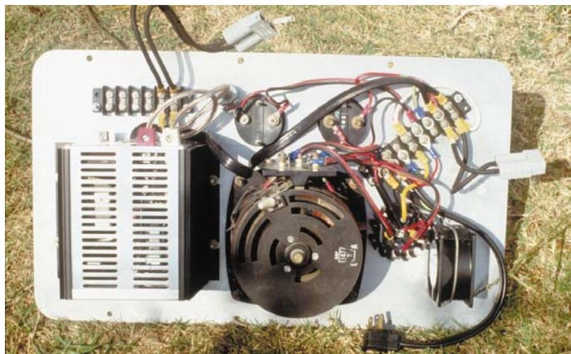
The Variac (right) and DC-DC converter (left) are panel-mounted. Use terminal strips for in/out power and instruments. Once installed, a cooling fan helps dissipate heat in the closed interior
