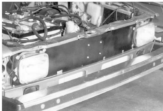
Air also finds its way into the engine compartment from below. Since we no longer need constant access for oil changes, we can bellypan the engine compartment. This is also a good idea for protecting the motor from dust, gravel, road splash, and winter road salt and sand.
