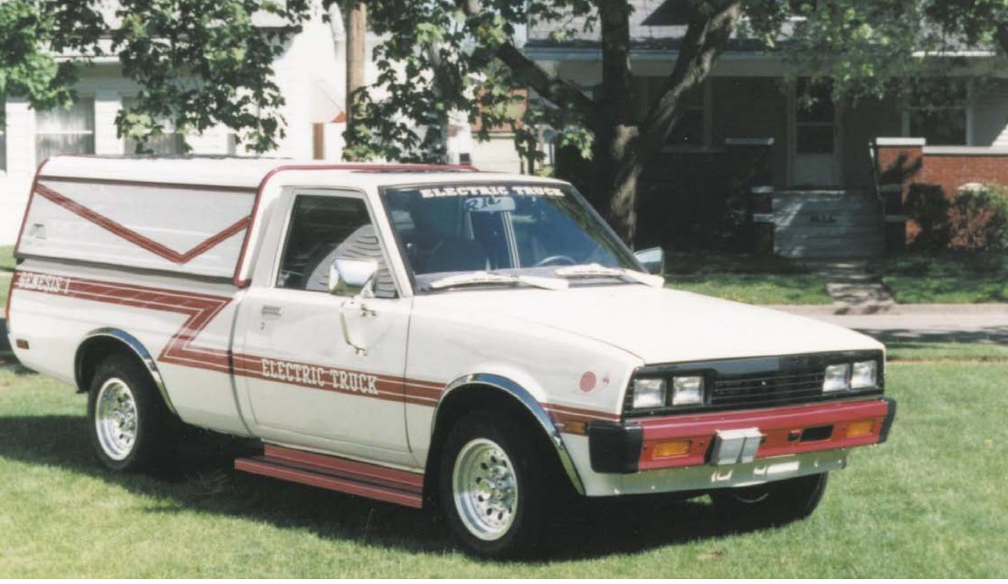
Above: Mark Parthe converted this 1984 Dodge D50 pick-up to run on electric power. The cost of the conversion was \$8000, including the used truck. Range is 75 miles and this truck has logged 8200 trouble-free miles since its conversion.
