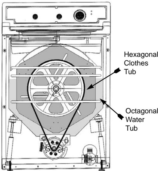
pumping action which forces the water through the clothes basket and agitates the clothes. The System 2000 spins at a higher RPM than most agitator washers. Faster spin cycles extract more water which leads to less drying time.
