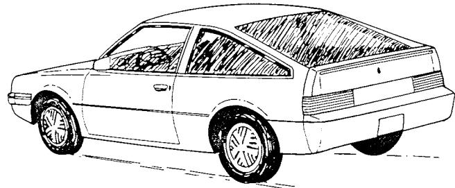
Above: A fastback body-style is more aerodynamic than a squared-off rear window and trunk.
