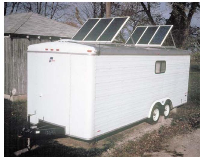
Above: The exterior of the portable solar-powered workshop with PV laminates raised and ready.
