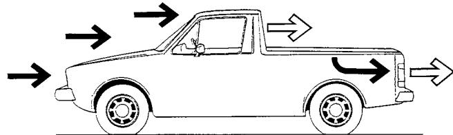
Above: Aerodynamic drag includes positive air pressure (black arrows) and negative air pressure or partial vacuum (white arrows).
