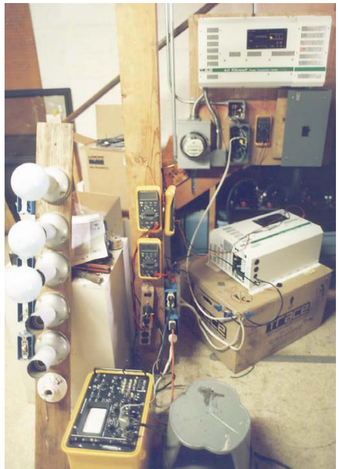
Above: Our testing jig for the Trace SW4024. We had to build an entire 120 vac distribution setup in order to test this inverter at full power (4000 watts). The 4024 on the wall is powering Bob-O's house, while the 4024 on the floor is undergoing testing. Note the Fluke 87s (hanging on the beam) and the oscilloscope (sitting on the floor).
