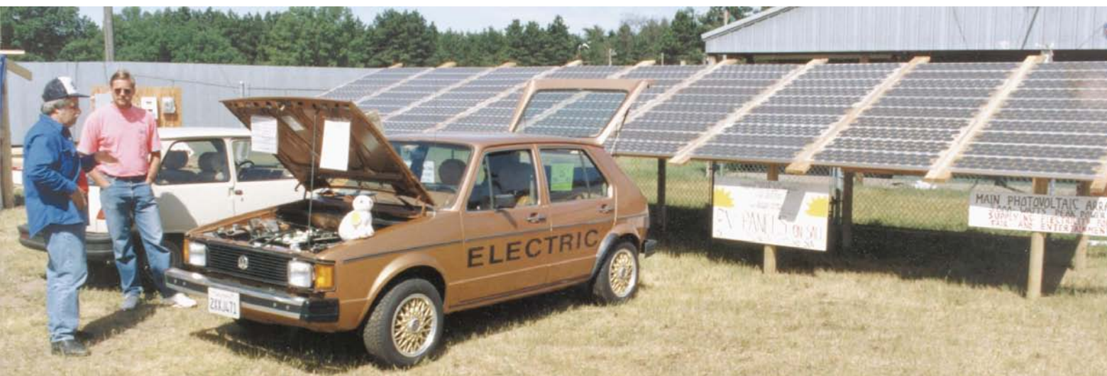
Above: It takes a solar array about the size of a household roof to charge an electric passenger car. Photo by Shari Prange
