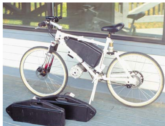
A center module houses controller and charger. Sealed batteries are wired into two fast-exchange saddlebags.
