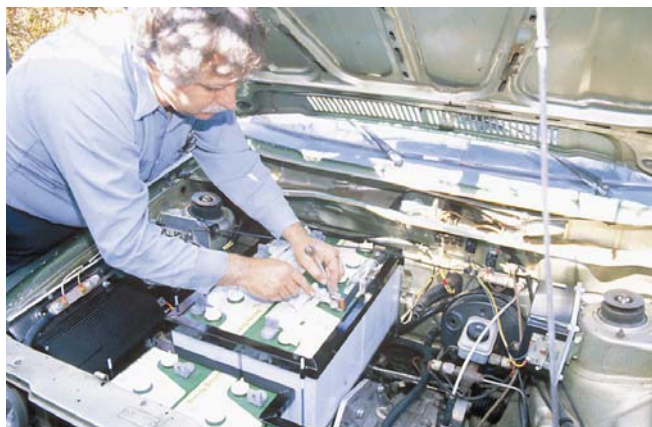
Above: Keep the electrical connections on the batteries tight and bright. Photo by Shari Prange
