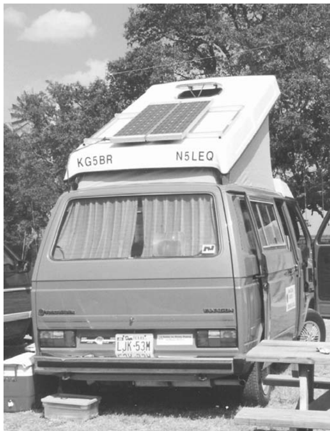
Above: "Sunflower," a 1984 VW camper, shows off the PV array on its tilt up roof.
