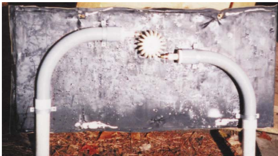
Above: A close-up view of the pelton wheel (5 inches in diameter) and the two 2 inch sweeps that end in improvised 5/16 inch nozzles.
