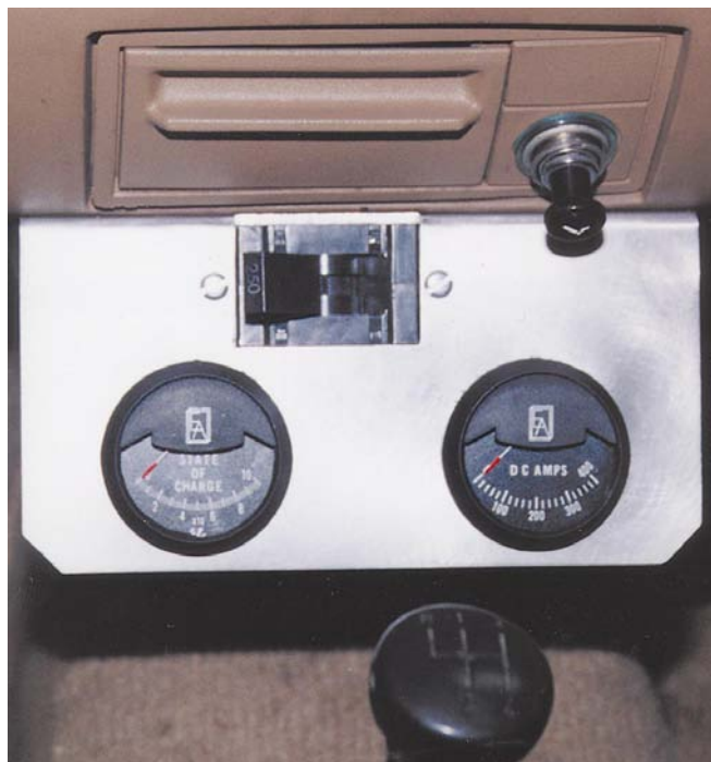
Above: The gauges and circuit breaker shared a common mount on the lower edge of the dash.
