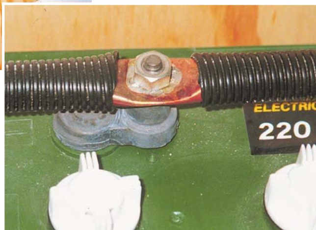
Below: A close up of the copper bus bar showing the wire loom covering and tinned area for better contact.
