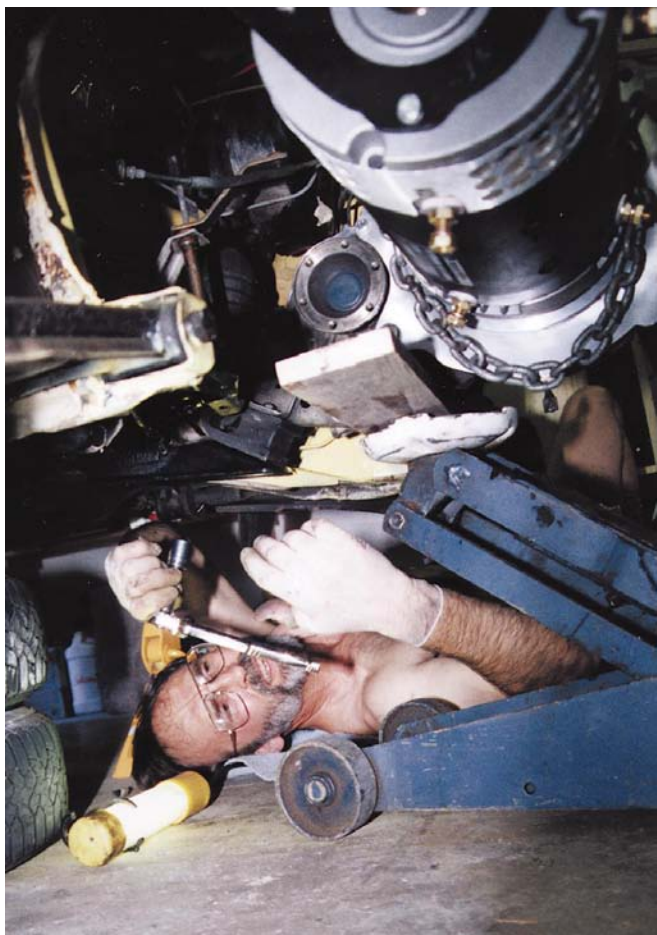
Above: Preston works under the car, bolting the motor and transmission into place.
