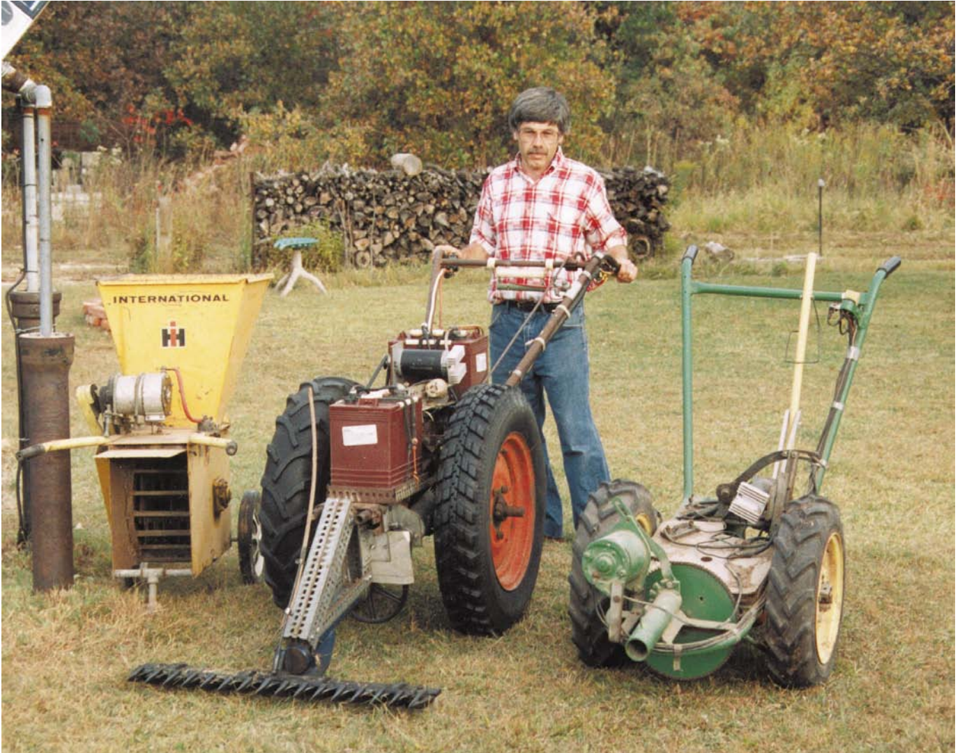
Above: The author with the electric David Bradley walking tractor. On the left is a compost shredder converted to 12 V and on the right is a home built 12 V rotary tiller.
