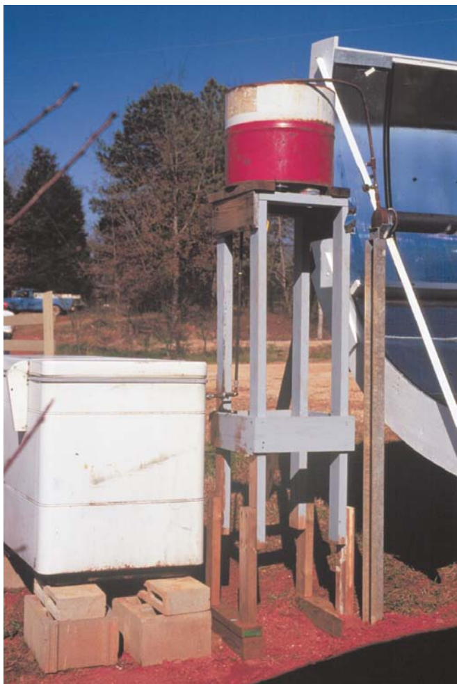
Above: Detail of the condenser bath, containing the condenser coil, and the icemaker box below.
