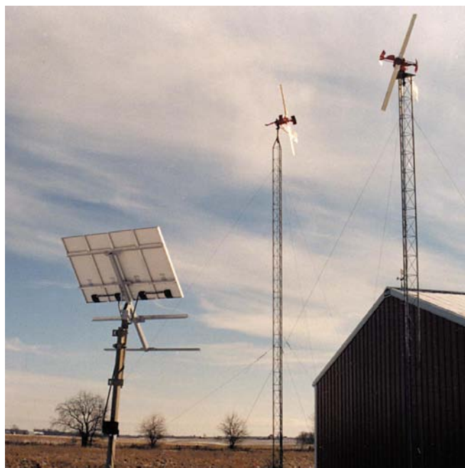
Above: Two 450 Watt Winco generators provide power for the shop. The PV mount has room for four more Siemens PC4 photovoltaic panels.
