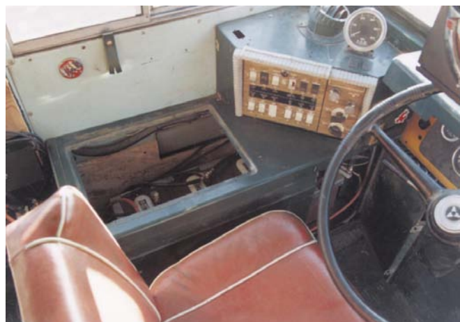
Above: The four Trojan T-105 batteries ride in a box under Rob's left elbow.
