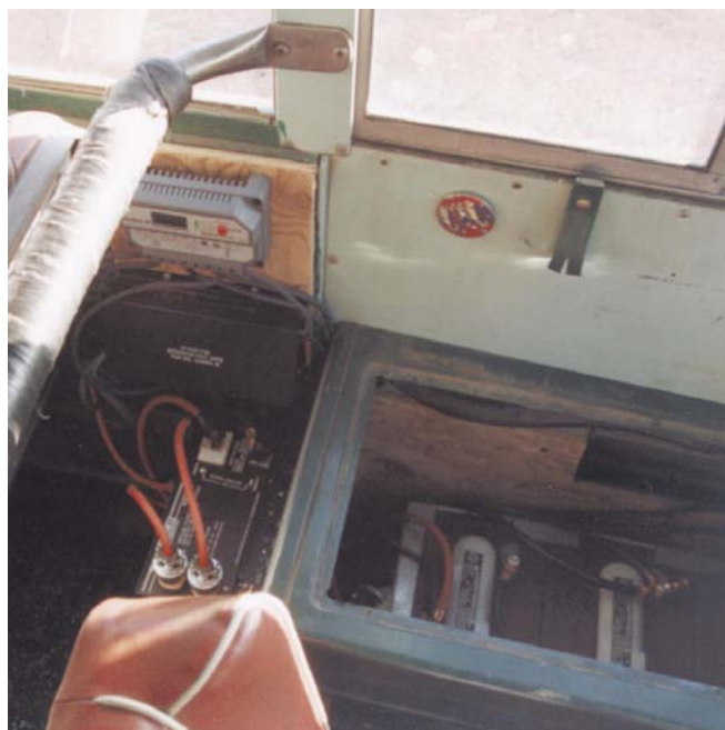
Above: Another view of the charge controller, inverter and batteries nestled to the left of the driver's seat.
