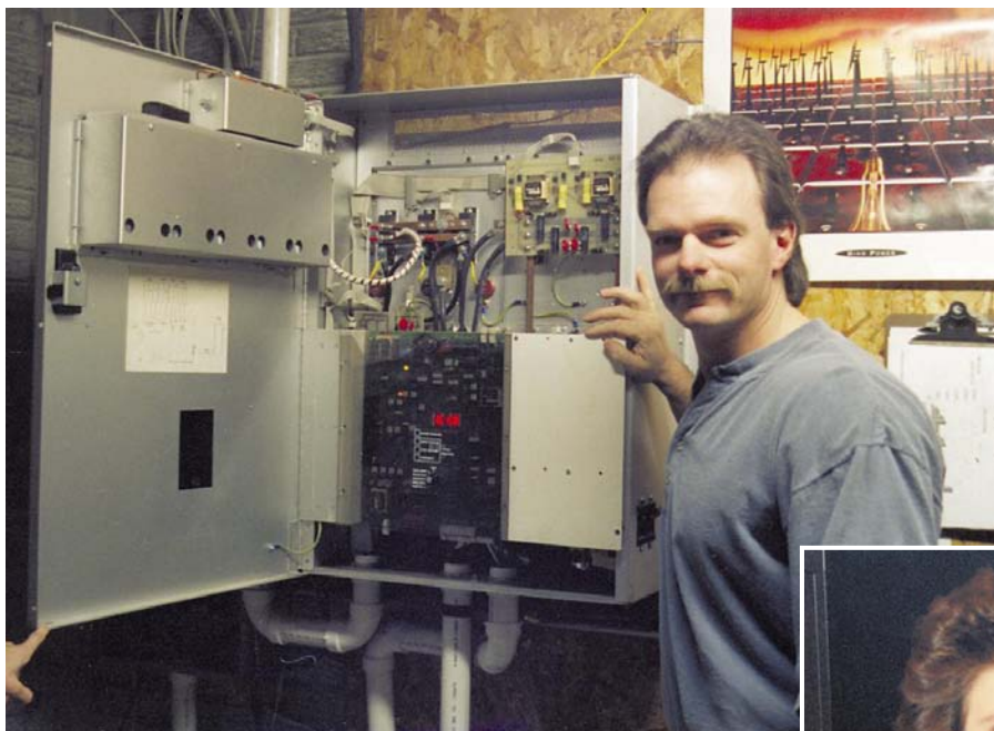
Left: Dan Whitehead shows off the inside of the Jacobs intertie inverter which converts 3-phase wild ac into single-phase 240vac.
