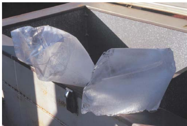
Above: About ten pounds of ice are created in one cycle of ammonia evaporation / condensation.
