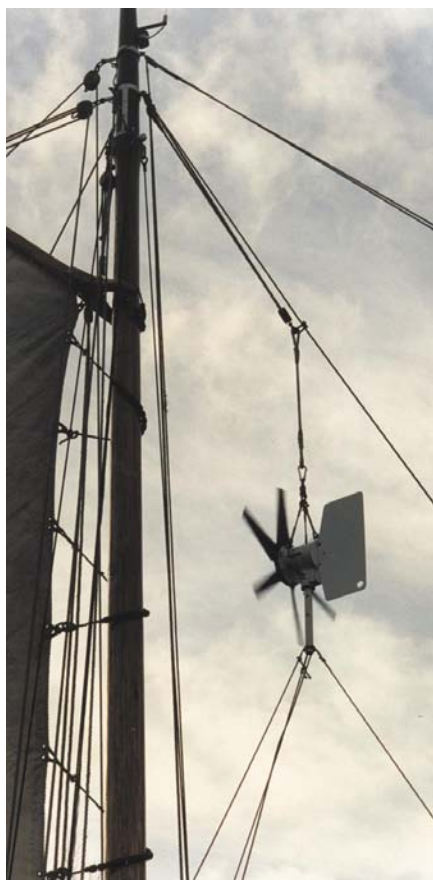
Above: The Ampair hoisted into "flying" position hangs from the foresail sheet in the triangle between the mast and the forestay.
