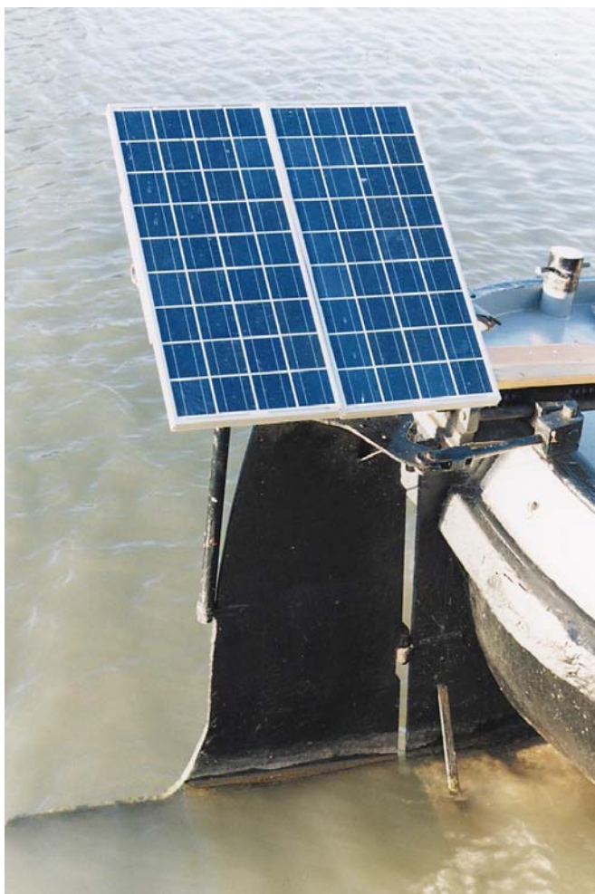
Above: The Kyocera modules are mounted on the rudder post keeping them out of the way of lines and other activity on deck.
