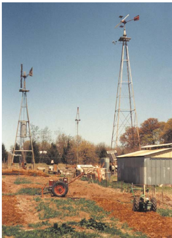
Above: The tractor is parked and its batteries are supplying power for the rotary tiller. In the background is the wind generator, the PV panels, and the water pumping windmill.
