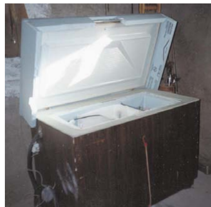
Right: NovaKool unit & extra insulation installed in an old chest freezer.
