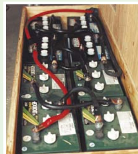
The batts: eight of the sixteen 220 amp hour batteries in Sun Chaser's hold.
