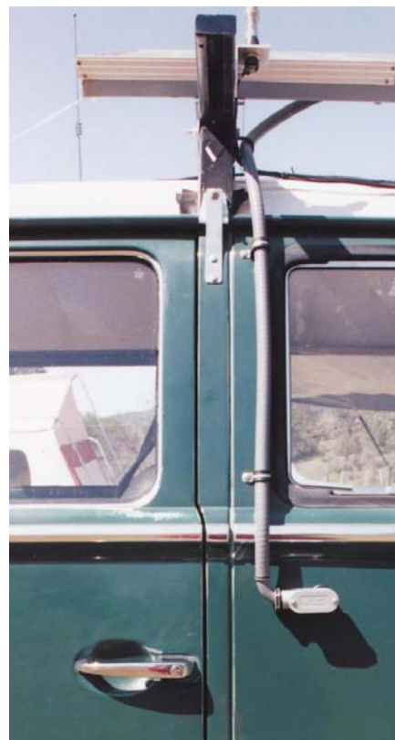
Above: A close-up view of the non-metallic flexible conduit and the bulkhead fitting into the bus.
