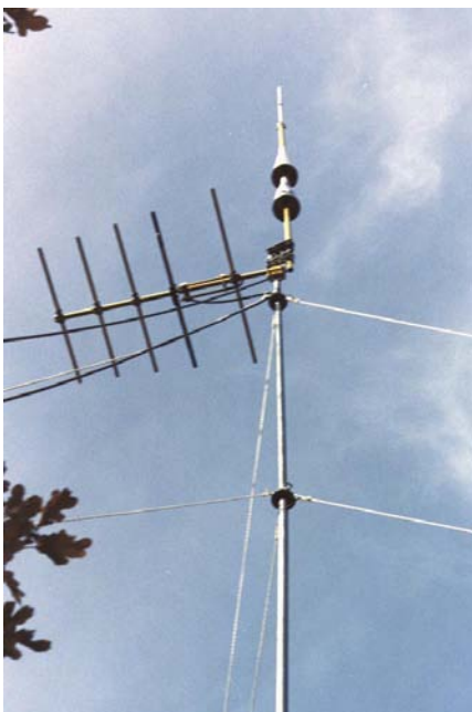
Left: Custom made Scala antennas are built to match the radiophone's frequency. The antenna on top of the mast is for 2 meter ham use.
