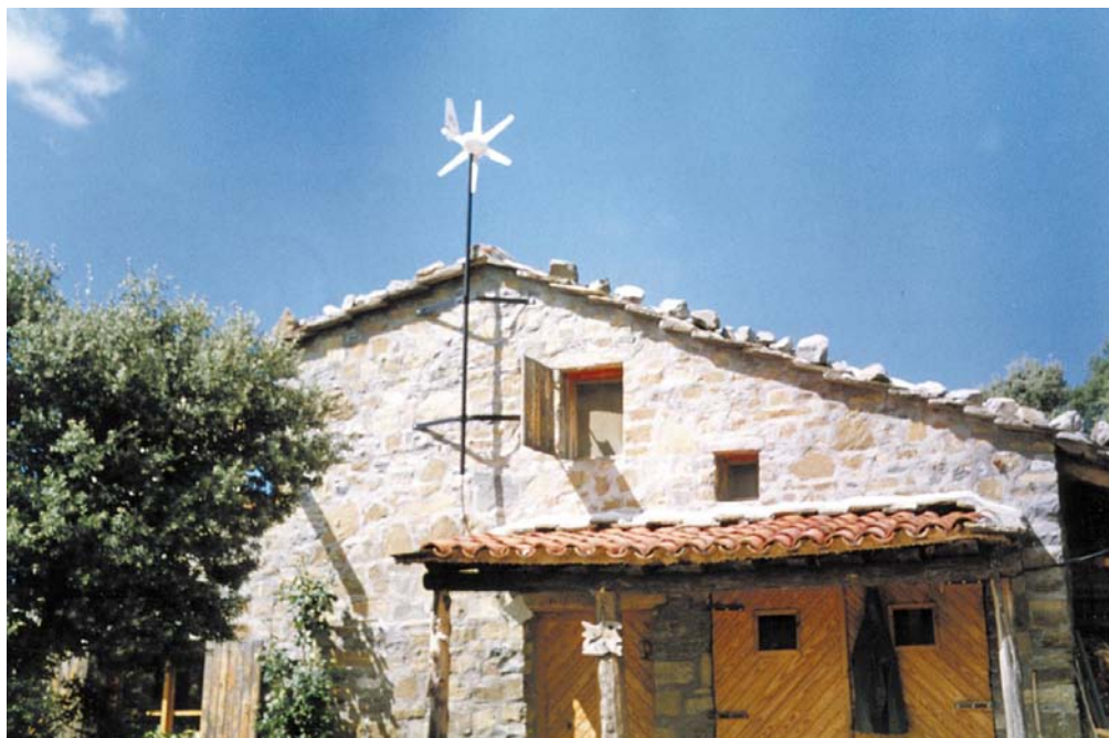
Above: An 80 Watt Rutland converts the turbulent Pyrenees winds to additional power during periods with little sun.
