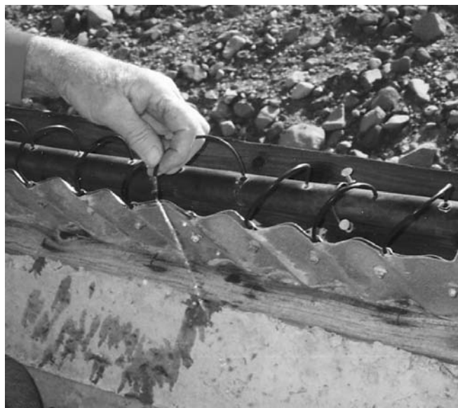
Above: Drip hose in action. Hose is tucked between pairs of corrugated metal sheets, and water gets heated as it runs down.
