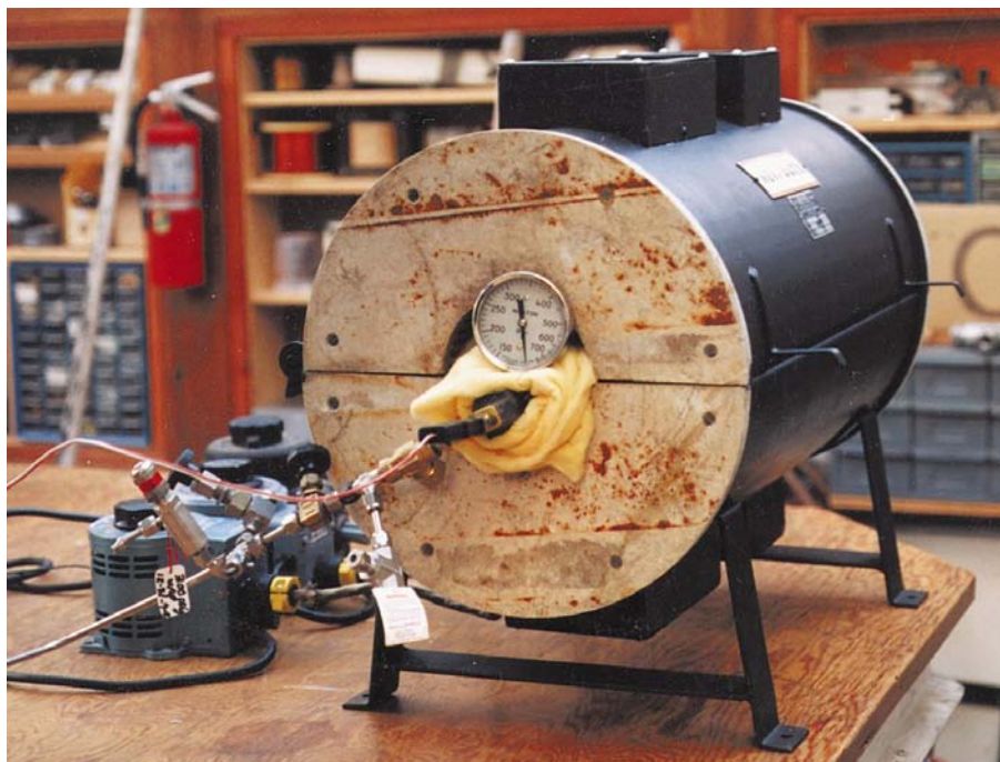
Above: Electric tube furnace ready for activation of MH cylinders.
