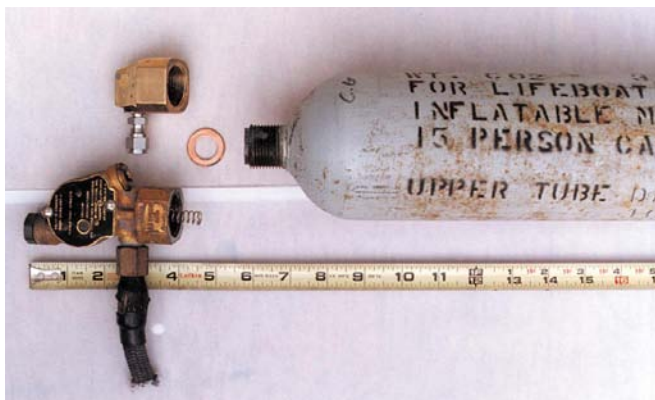
Left: CO 2 cylinder to be converted to H 2 storage in metal hydride.
