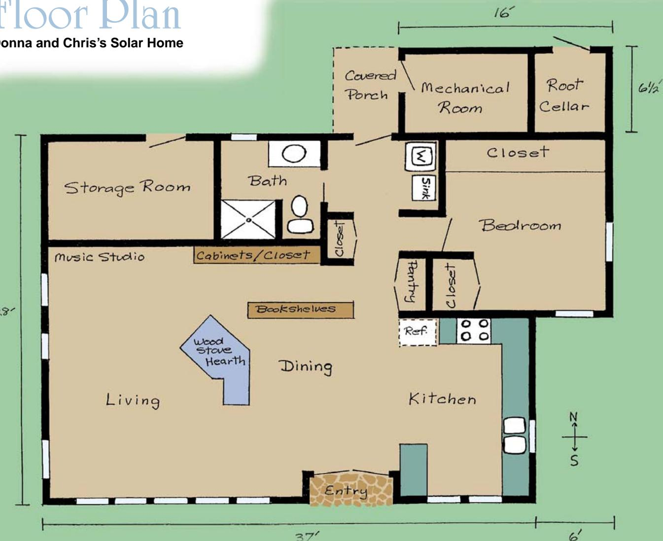
south side of the house to take maximum advantage of the solar warmth and light. Note also that the north side of the house is partially buffered by the unconditioned spaces and the bedroom closet.
