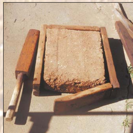
Above: Hinged form and pounding mallet.
