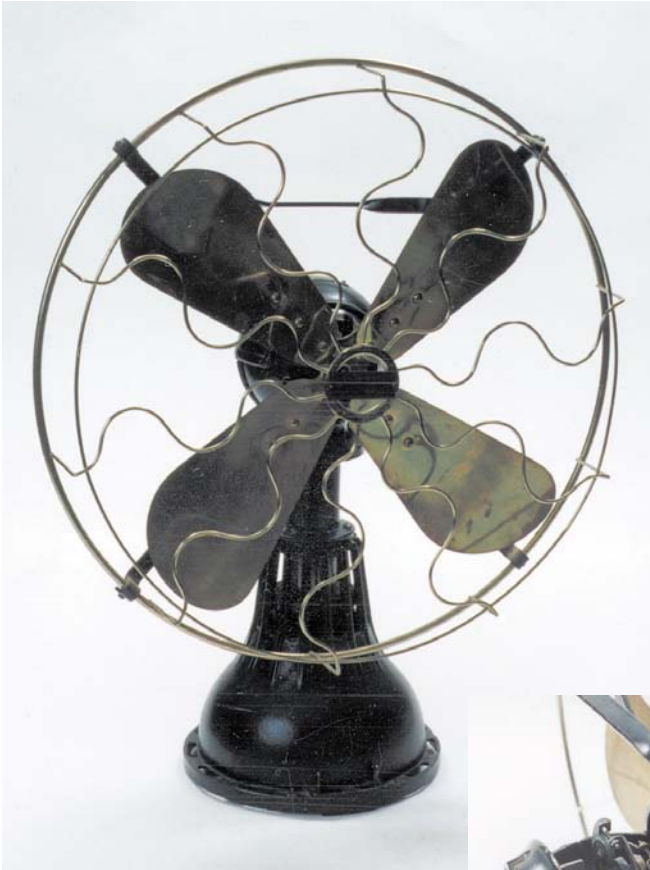
Above: The 1906 Lake Breeze fan runs on alcohol.
