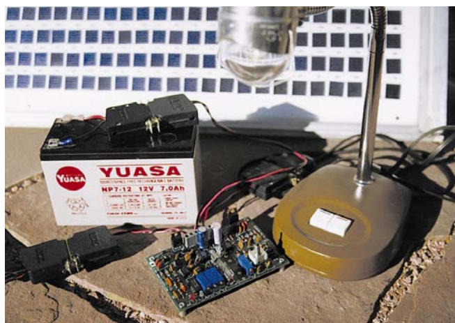
Above: Charge controller circuit board in action.
