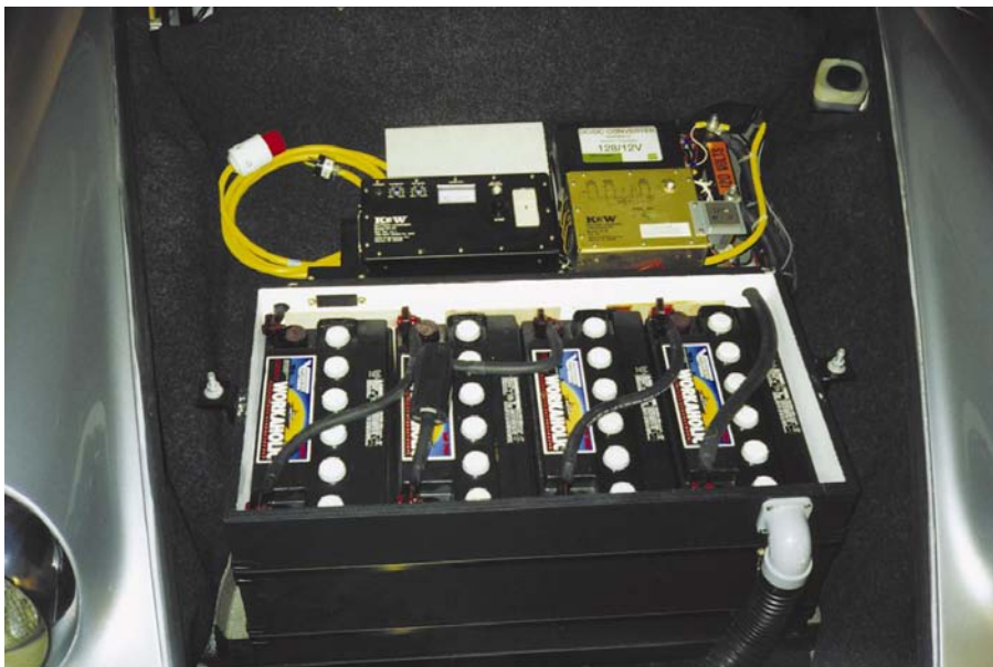
Below: More batteries, charger, and DC/DC converter in the nose.
