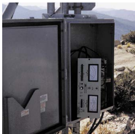
Left: The translator, in a weather tight box, is mounted on the PV / antenna structure.
