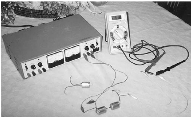
Above: Simple motor test rig. Batteries can be used instead of a power supply.
