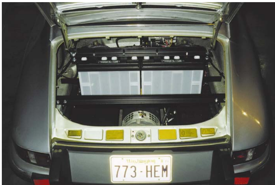
Above: Rear batteries in the engine compartment with a glimpse of the Advanced DC motor beneath.
