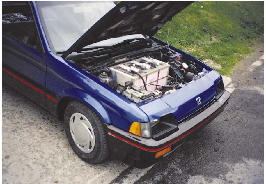
Above: Reserving the central area under the hood for batteries will make your conversion easier.
