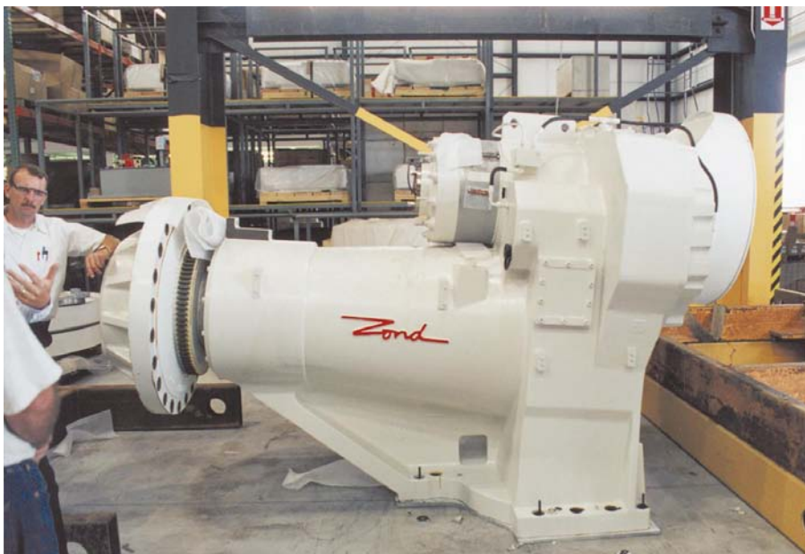
Above: The heart and soul of the Zond machine, its integrated gearbox.
