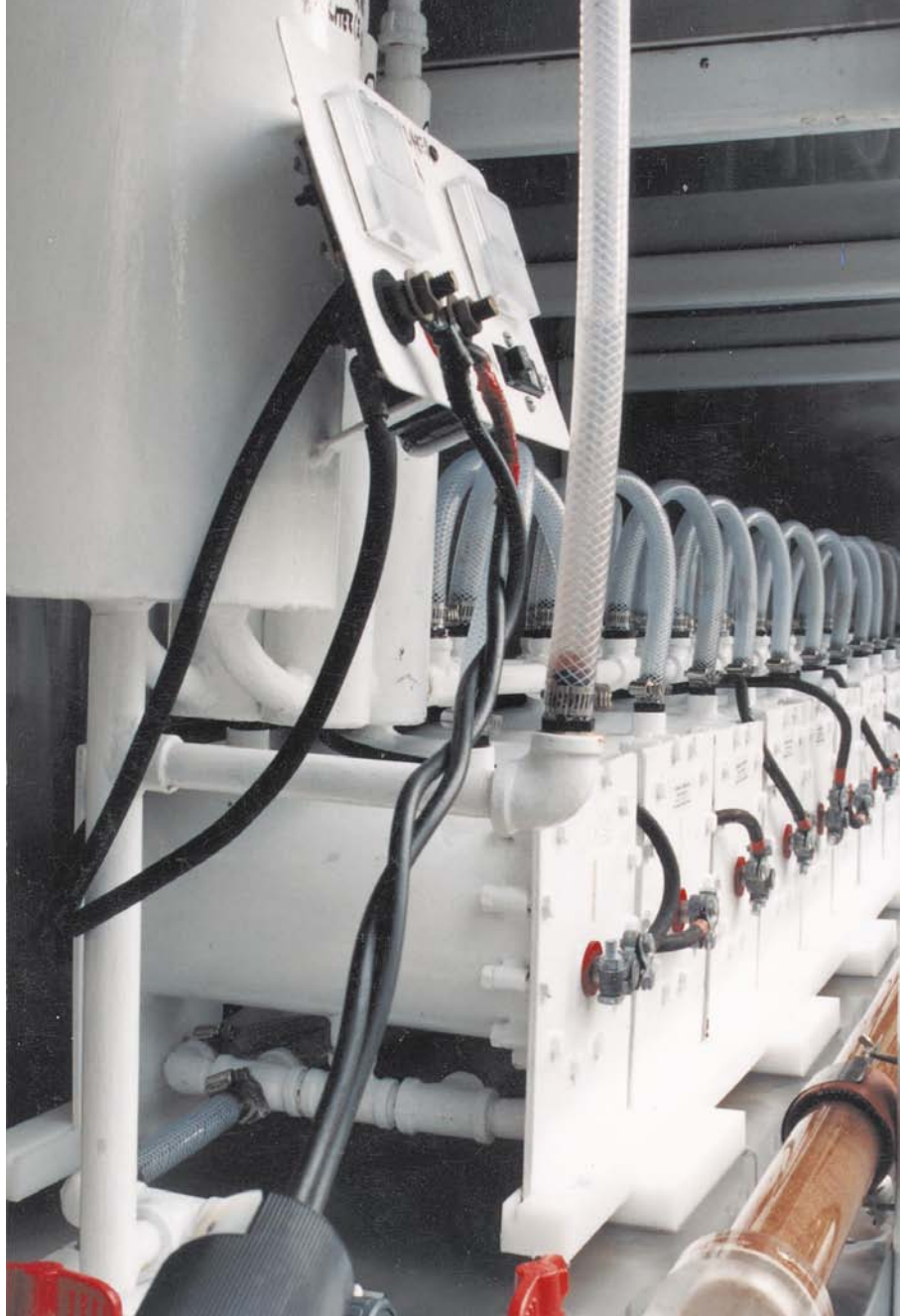
Above: Electrolyzers driven by photovoltaics.
