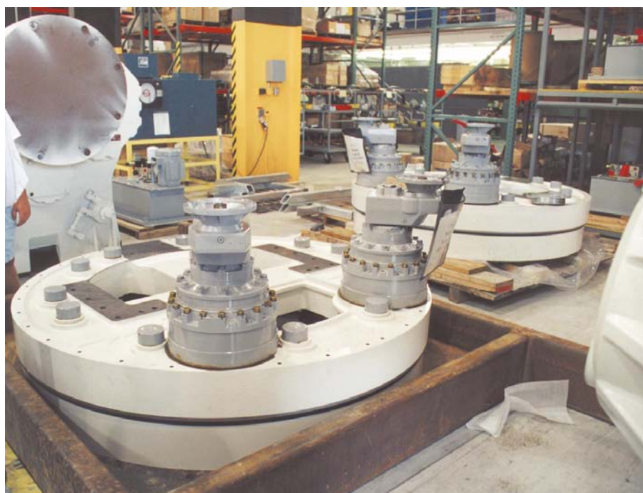
Below: The tower-top collar and the servos that control yaw.
