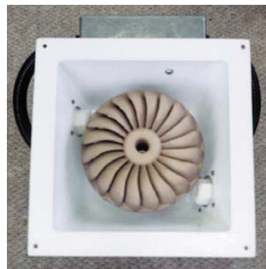
Above: The underside of the Turgo turbine.
