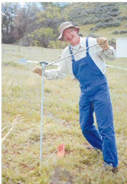
Above: The screw anchors can be driven by hand.
