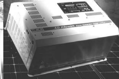
TRACE Sine Wave 4000 Watt Inverter Charger. 10,000 Watt Surge Power with 2800 Watt Charger. Fully programmable, including control of generator and relay closures. Stackable for double the power.
