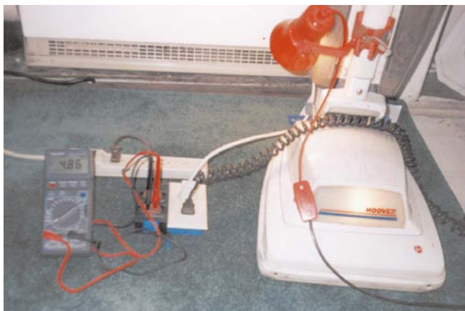
Measuring volt-amperes on the vacuum cleaner, using the clip-on incandescent light as the resistive component.
