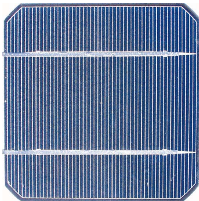
A screen-printed photovoltaic cell.
