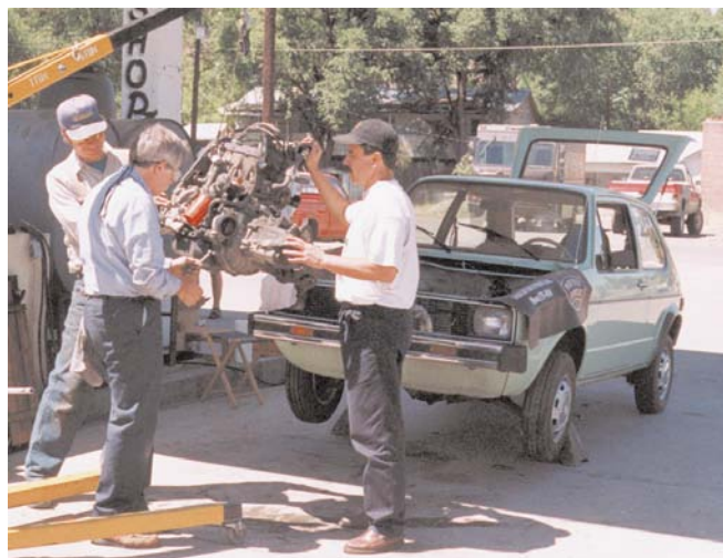
Hoisting out the internal combustion engine.
