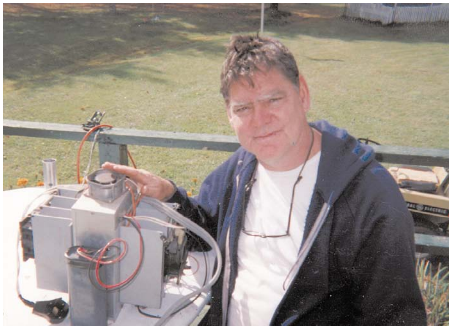
John with his home-built, 6 KW, 120 VDC in, 120 VAC out square wave inverter. It draws 3 watts at idle and is 99.5 percent efficient with a 1,000 watt load.
