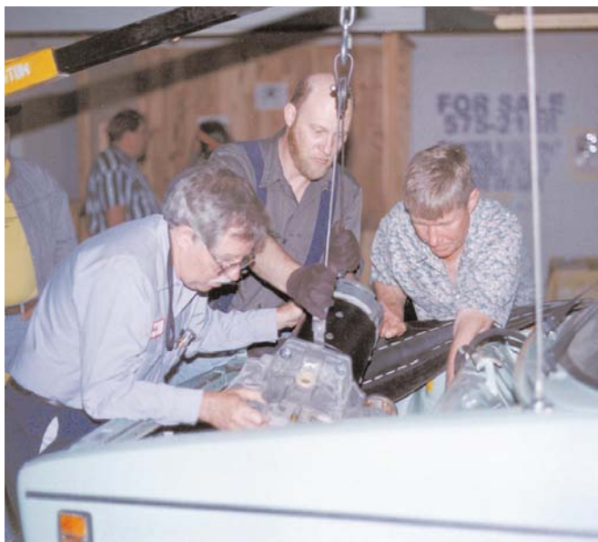
Lowering the new electric motor into place.
