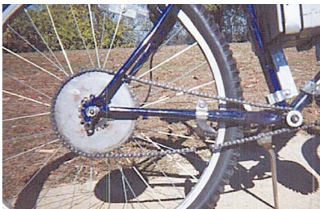
Drivetrain from the 13 tooth sprocket on the bottom bracket spindle to the 60 tooth sprocket on the rear hub.
