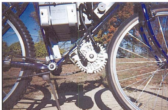
The Scott Motors 24 VDC PM motor and two PowerSonic 28 AH batteries can drive this bike to 30 mph.
