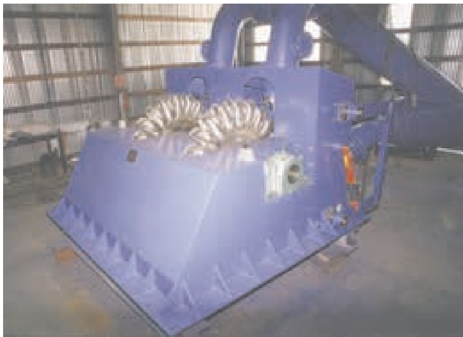
A large (1,400 KW) Canyon Pelton turbine with two runners and four nozzles, operating near Idaho Falls, Idaho.
