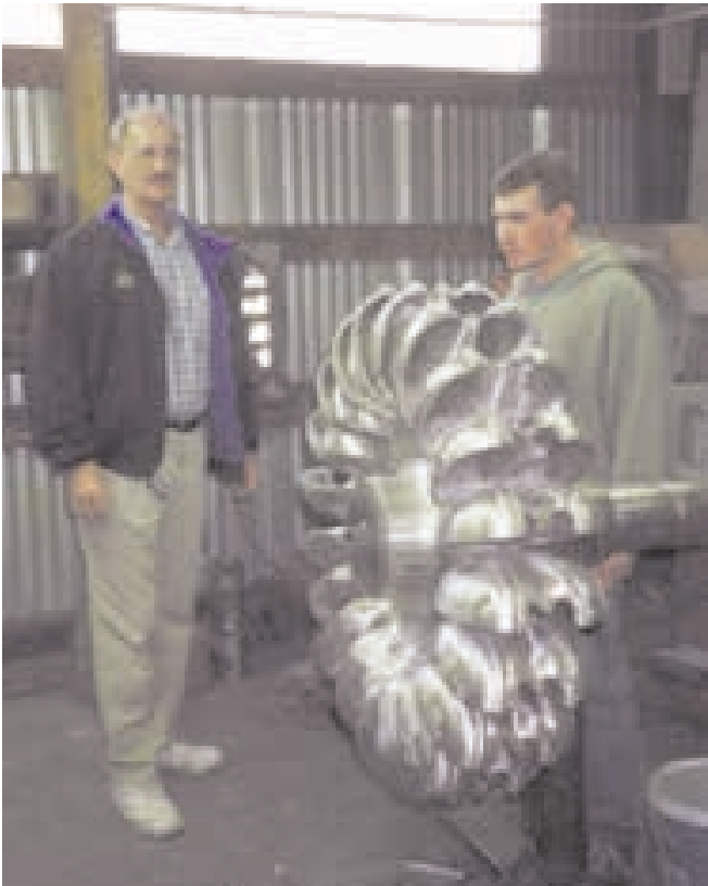
Dan and a Canyon employee with a Pelton wheel on the grinding and polishing stand.
