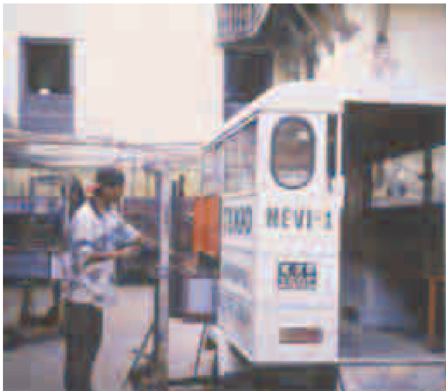
A working EV's daily ritual. Swapping in the second set of batteries at midday.
