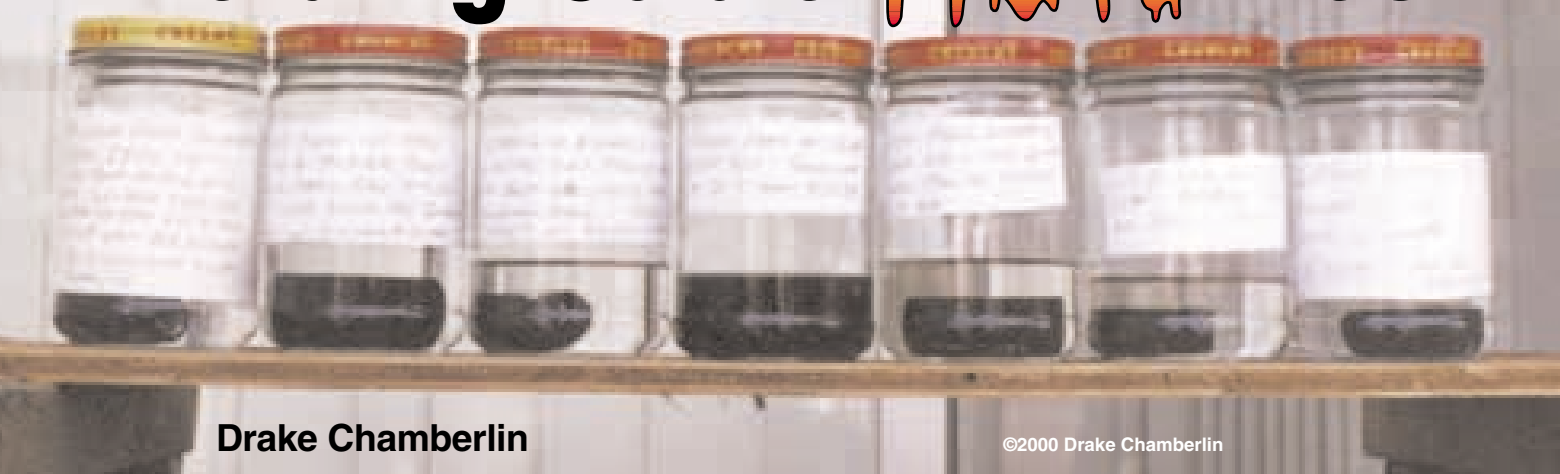
Cable specimens soaking in battery acid.
