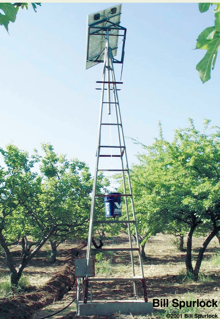
The author's water-powered PV tracker.
