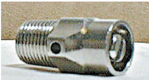
Coin vents at high points in the system allow easy release of trapped air bubbles.
