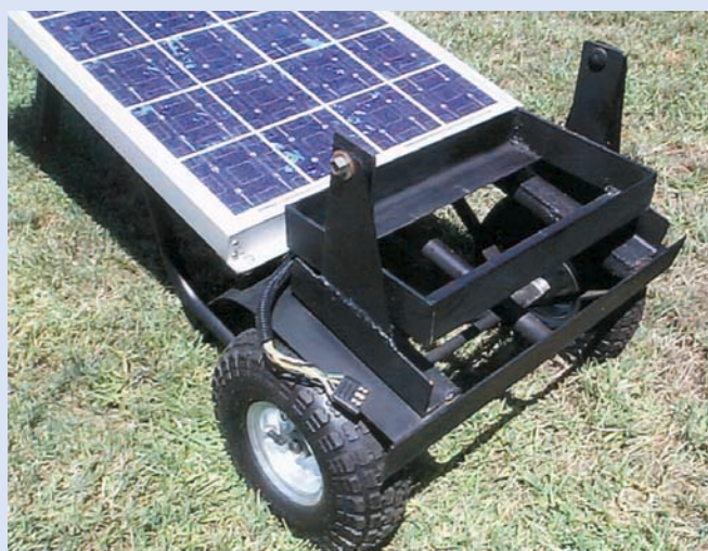
This homemade battery cradle keeps the flooded lead-acid battery level so electrolyte doesn't spill.
