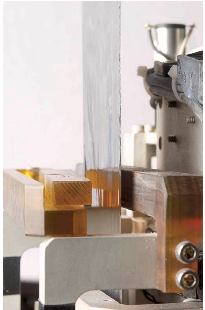
A ribbon of crystallized silicon 81 mm wide and 1/4 mm thick is pulled from the molten pool at 16 mm per minute.
