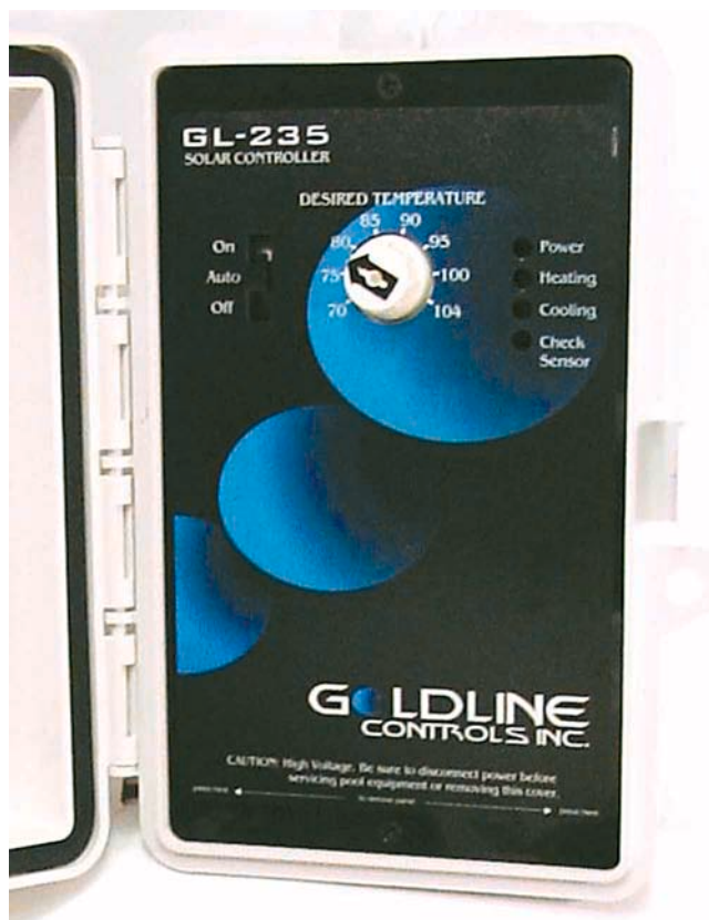
A differential pool controller senses pool and solar collector temperatures and controls the diverter valve appropriately.
