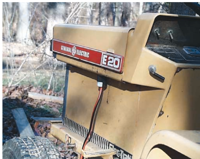
The solar-electric charging system hooks up to the Elec-Trak's 36 volt accessory port.
