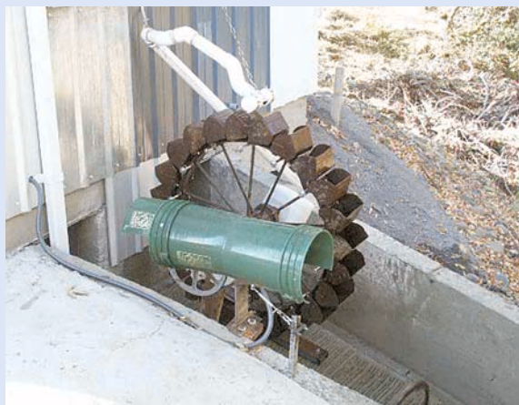
A small, 4 foot diameter water wheel was built using parts from an old feed mill.
