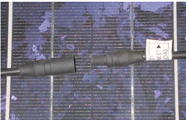
An MC (Multi-Contact) connector.
