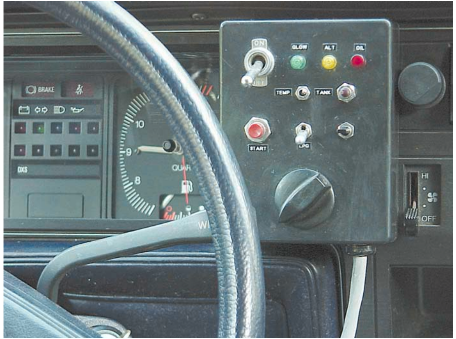
Pusher controls on the dash of the EV.
