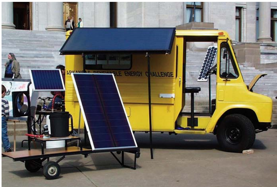
This 32-year-old postal van, which was converted to run on electricity, serves as a demonstration tool for various renewable energy technologies.
