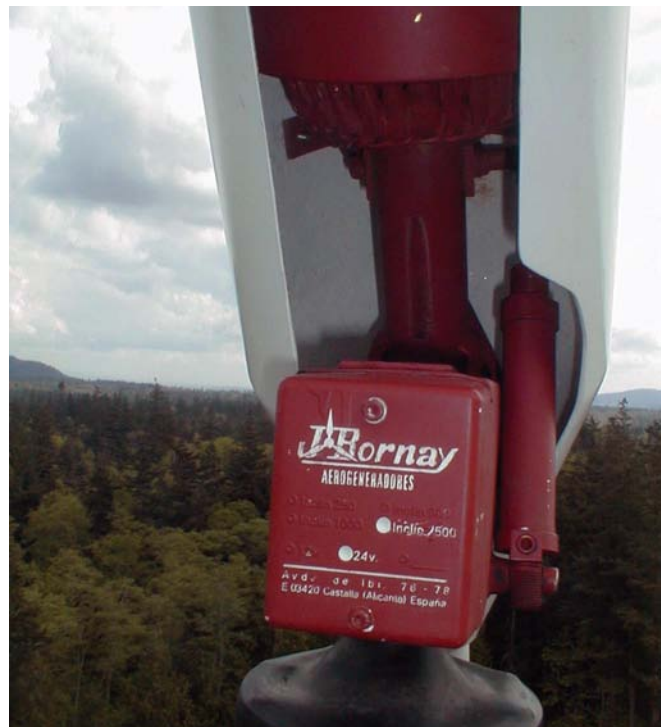
Bornay Inclín 1500 generator and shock absorber in governing position (tilted back).
