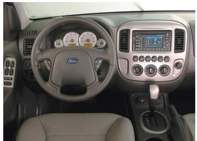
The cockpit with the color LCD screen that displays operating mode and continuous data on performance.
