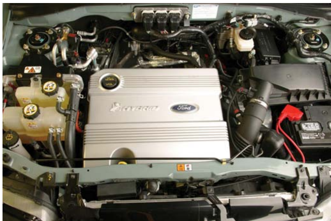
The 2.3 liter internal combustion engine only provides 133 horsepower—the electric motor adds 94 more.
