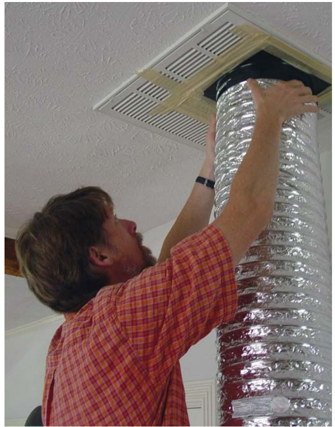
Connecting the Duct Blaster to a return duct in preparation for pressurizing the duct system.
