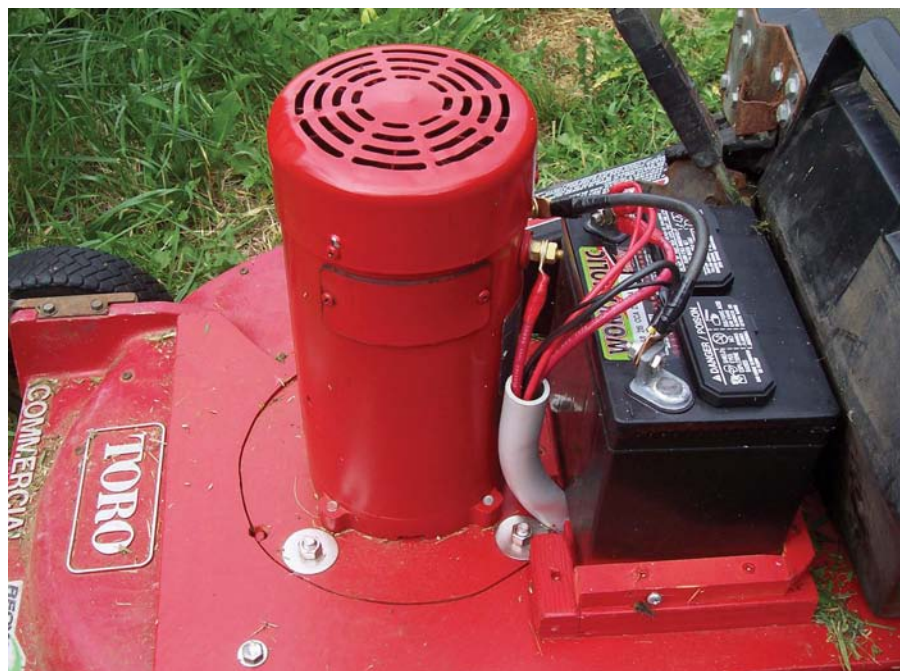
The new, electric Toro's motor and battery (with battery cover removed).
