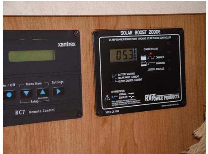
An RC7 Remote Control and SB 2000E charge controller monitor the system's performance.
