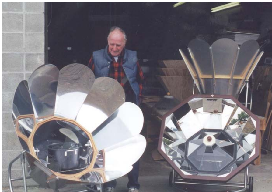
Solar cooking pioneer Sam Erwin designed the highly efficient Solar Chef, a solar cooker that combined the features of a box cooker and a parabolic reflector cooker.
