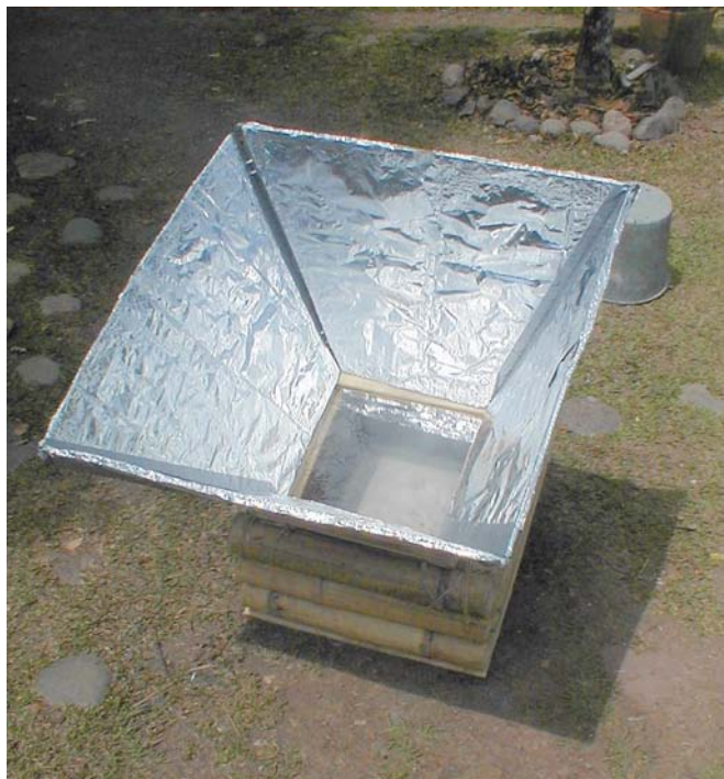
This homemade box cooker uses a bamboo oven box and foil-covered cardboard reflectors.
