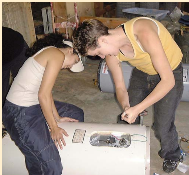
Amber Crowley and Keiko Suda assemble their first water heater tank-based biodiesel reactor at an East Bay biodiesel internship class.
