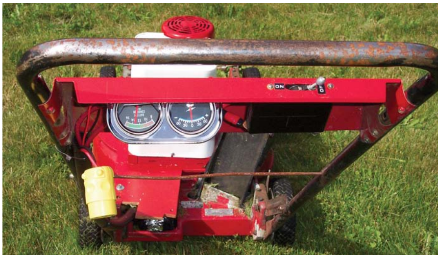
Every project needs meters! A voltmeter and ammeter are mounted on the mower. The mower plugs into a small PV system for charging.
