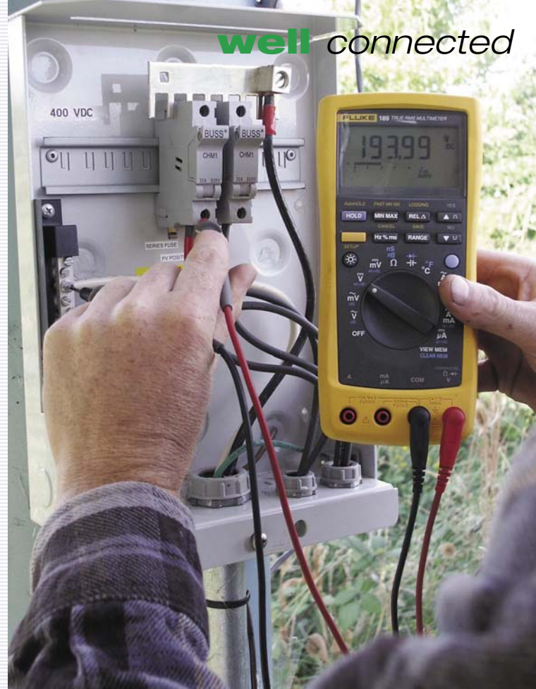
Using a digital multimeter to measure array voltage.
