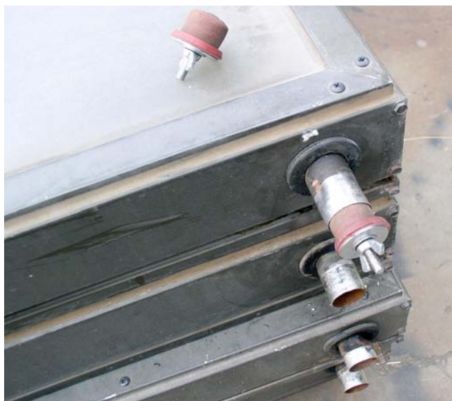
A temporary compression plug used to seal a header pipe port so the collector can be pressure tested.
