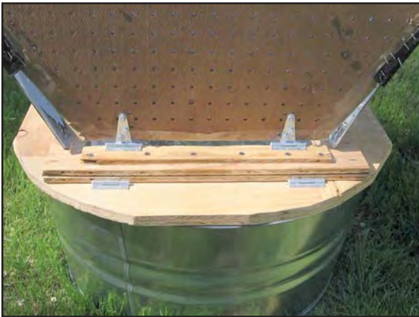
A close-up of the hinge placement and reflector attachment.
