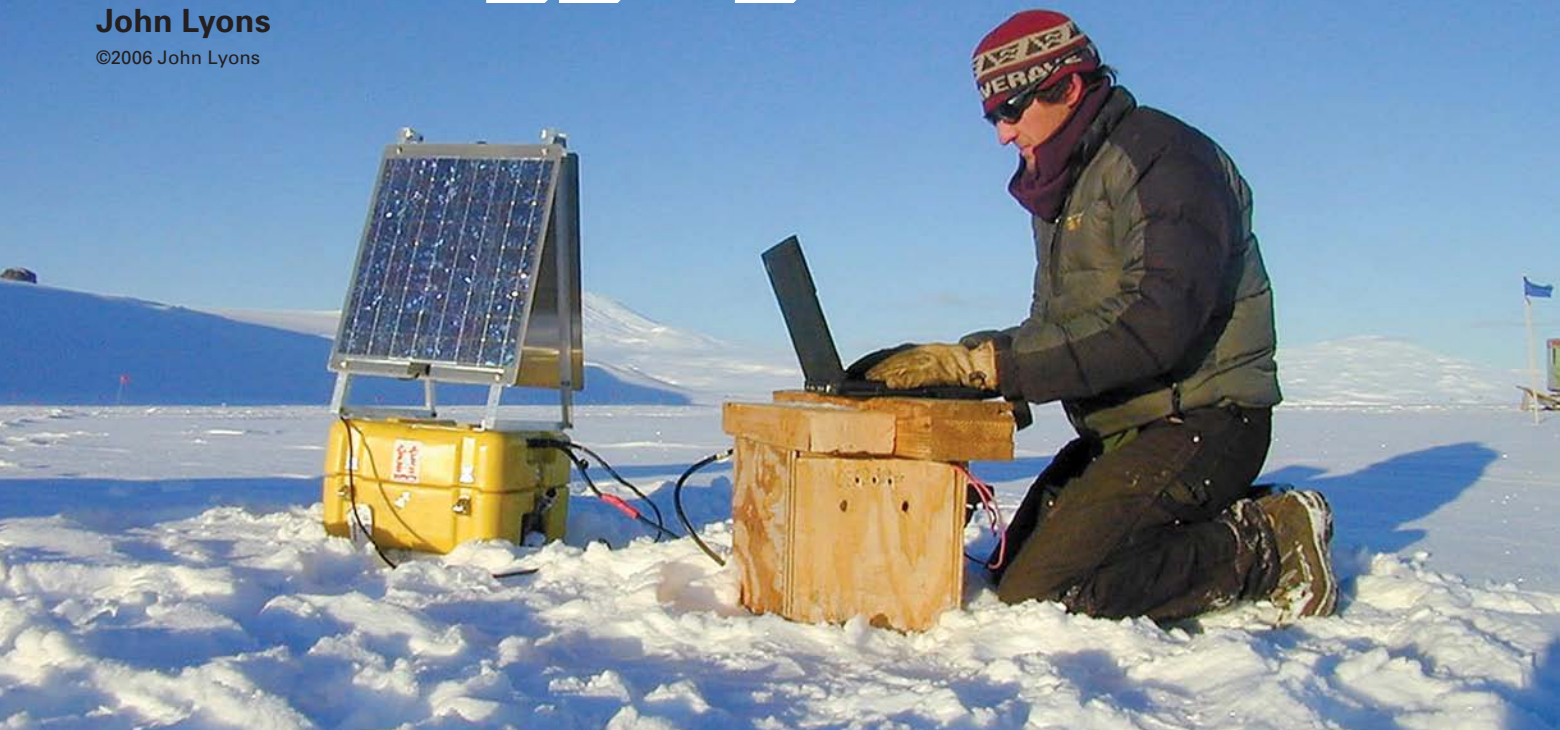
The author downloads performance data from a portable solar-electric system on the McMurdo Ice Shelf in Antarctica.
