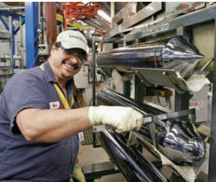
Measuring single-crystalline silicon ingots at the SolarWorld PV plant in Vancouver, British Columbia.
