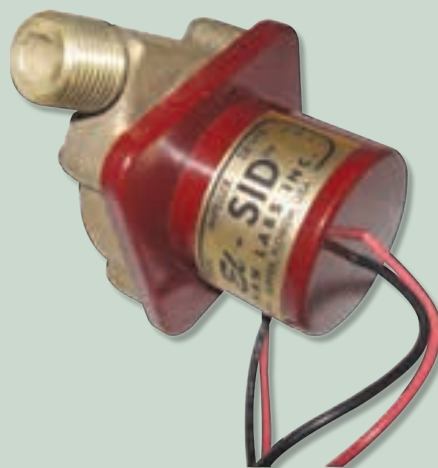
EI-Sid 10 PV, DC pump. Although it may run on a 10-watt PV module, this pump is usually coupled with a 20-watt module to make sure it starts in all applications.
