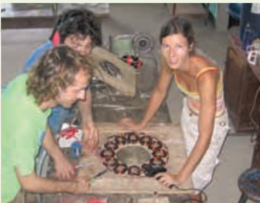
In the shop, blueEnergy team members test the stator (left) and set rotor magnets in resin (right).
