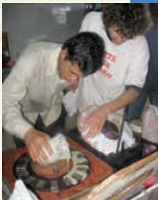
In the shop, blueEnergy team members test the stator (left) and set rotor magnets in resin (right).
