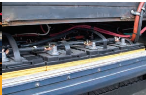
Assembling the interconnects and battery overcurrent protection. Far right: The neatly wired battery bank.
