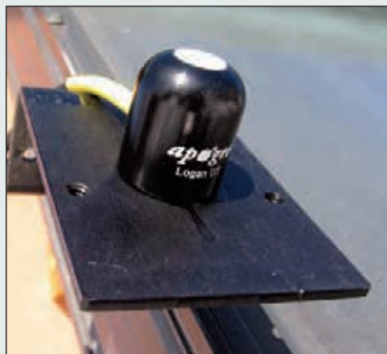
Solar irradiance is measured with a pyranometer.
