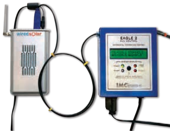
IMC Instruments's Eagle 2 differential controller works with a transceiver (above) to send system data to the Web (left).
