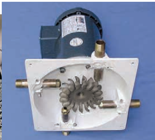
The Hi Power hydro unit matches a Harris Pelton turbine to an induction motor to generate wild three-phase AC at up to 480 V, and 3.6 KW.
