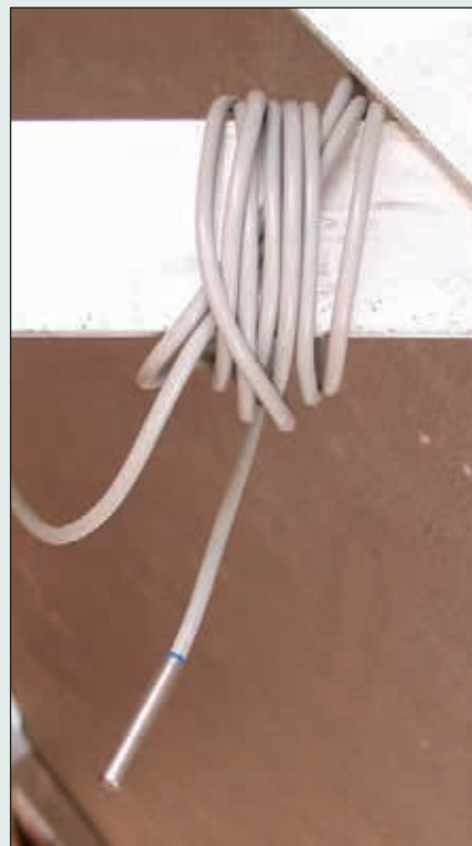
The ambient temperature probe hanging in the shade behind the collectors.
