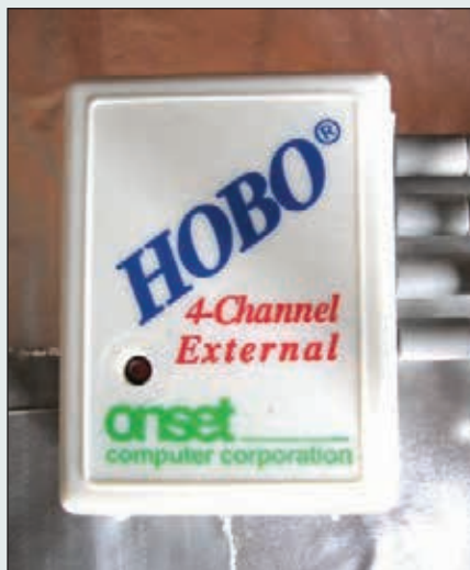
The data logger records three temperatures and irradiance.
