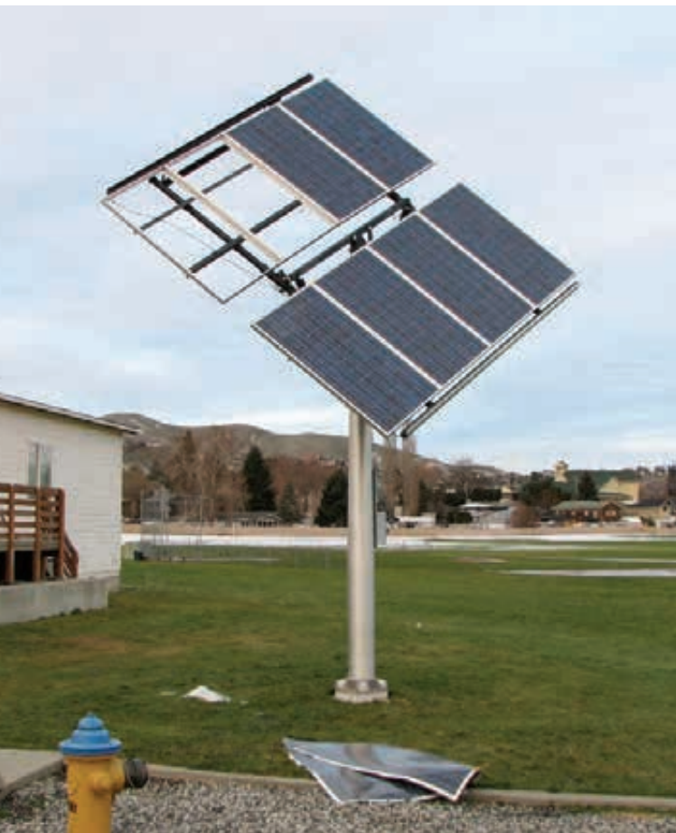
Extreme winds blew two laminates right out of their frames on this pole-mounted PV array.
