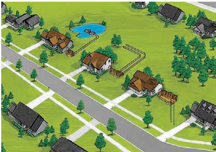
From left to right: A lake loop in a pond, a horizontal loop in filled-in trenches, and a vertical loop in bored wells.
