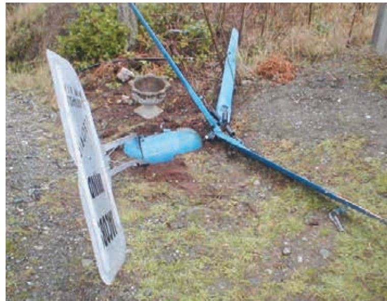
One loose bolt sent this direct-drive Jacobs wind turbine to the ground. The homeowner's insurance policy covered the turbine replacement.
