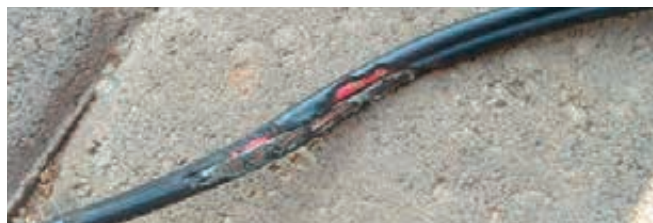
An abraded cable (in this case, rodent-damaged) can lead to shorts and malfunctioning systems.
