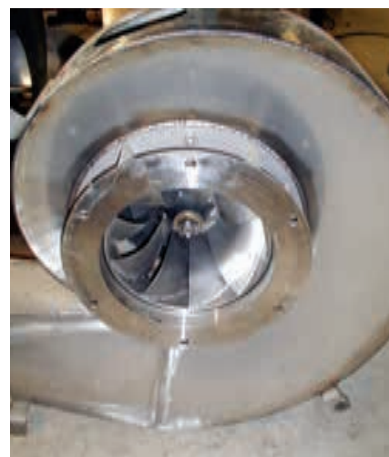
Below: The runner sits at the output of the scroll case in one of Ron's Nautilus turbines.
