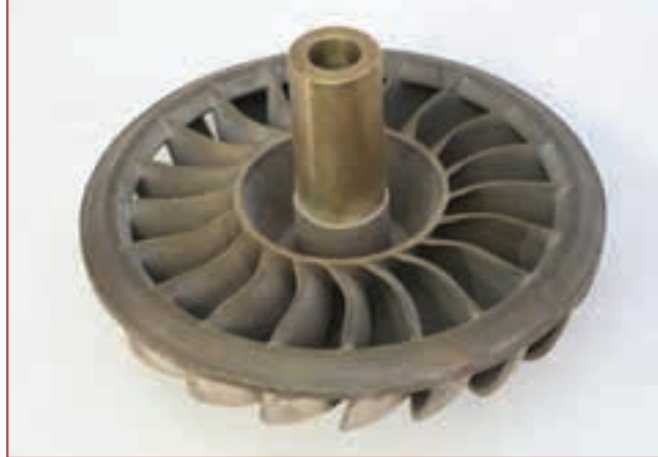
The design of the Turgo runner performs better with more flow than a Pelton runner, but is also a pressure-dependent design.
