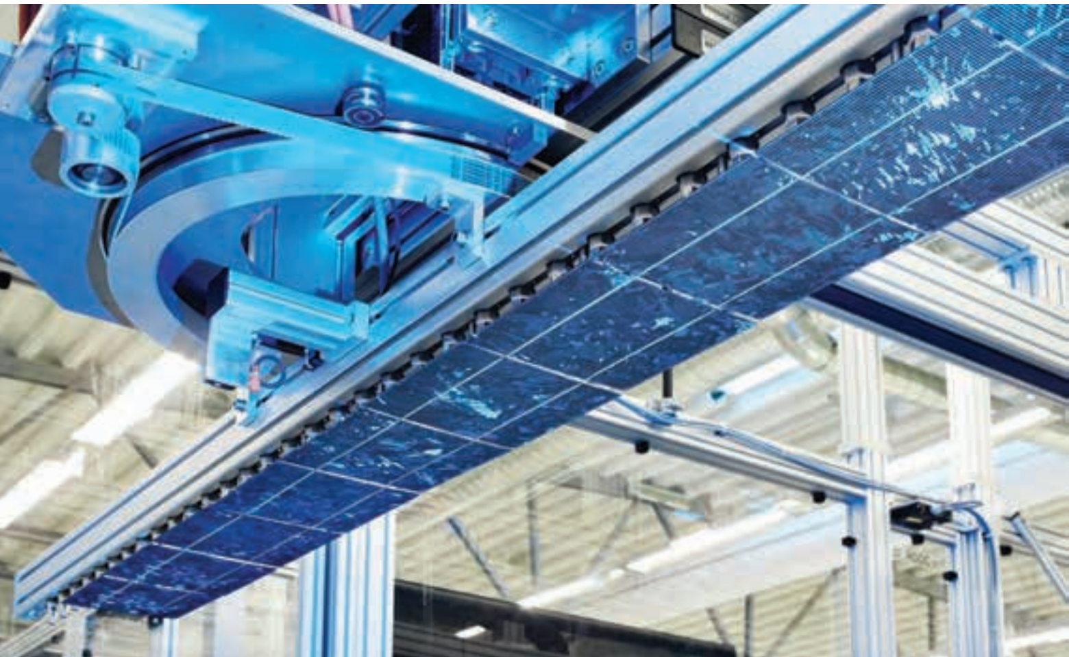
Above: A robot with pneumatic suction prepares to place a series string of cells.
