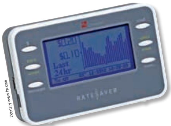
LS Research's RateSaver monitor displays energy use and related data in an easy-to-read, in-house display.
