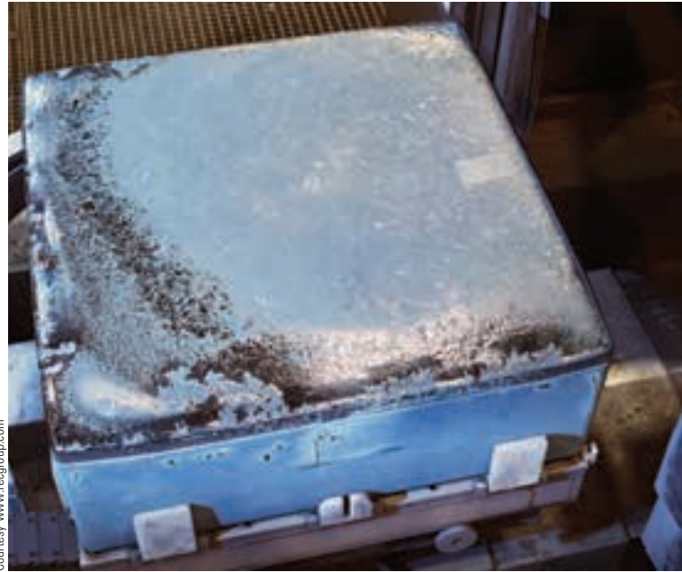
A poured multicrystalline ingot, ready to be sawn into cell-sized wafers.
