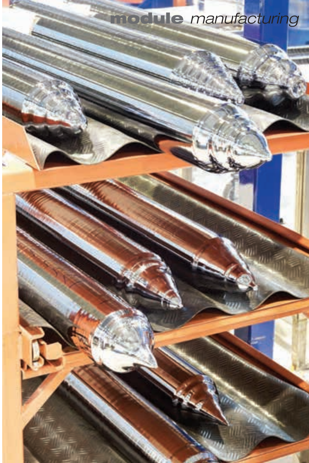
Monocrystalline boules created using the Czochralski process.
