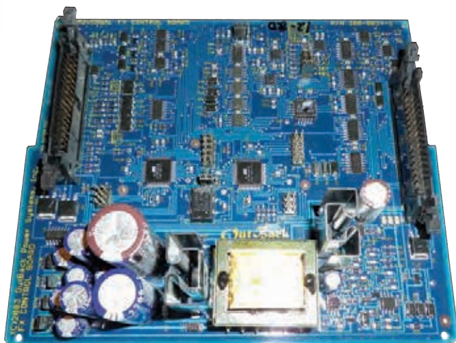
Inverter controllers can be complex computers, but in some cases they might be as simple as a single-chip logic circuit.
