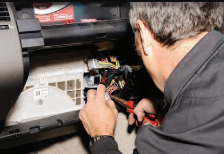
Technicians prepare the wiring behind the dash for the new "electric vehicle" switch.
