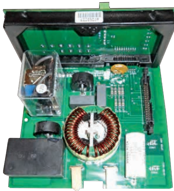
AC filters help smooth out the waveforms and reduce radio frequency interference.
