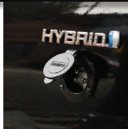
Above: The male AC receptacle and its cover are the only external signs of the installation.
