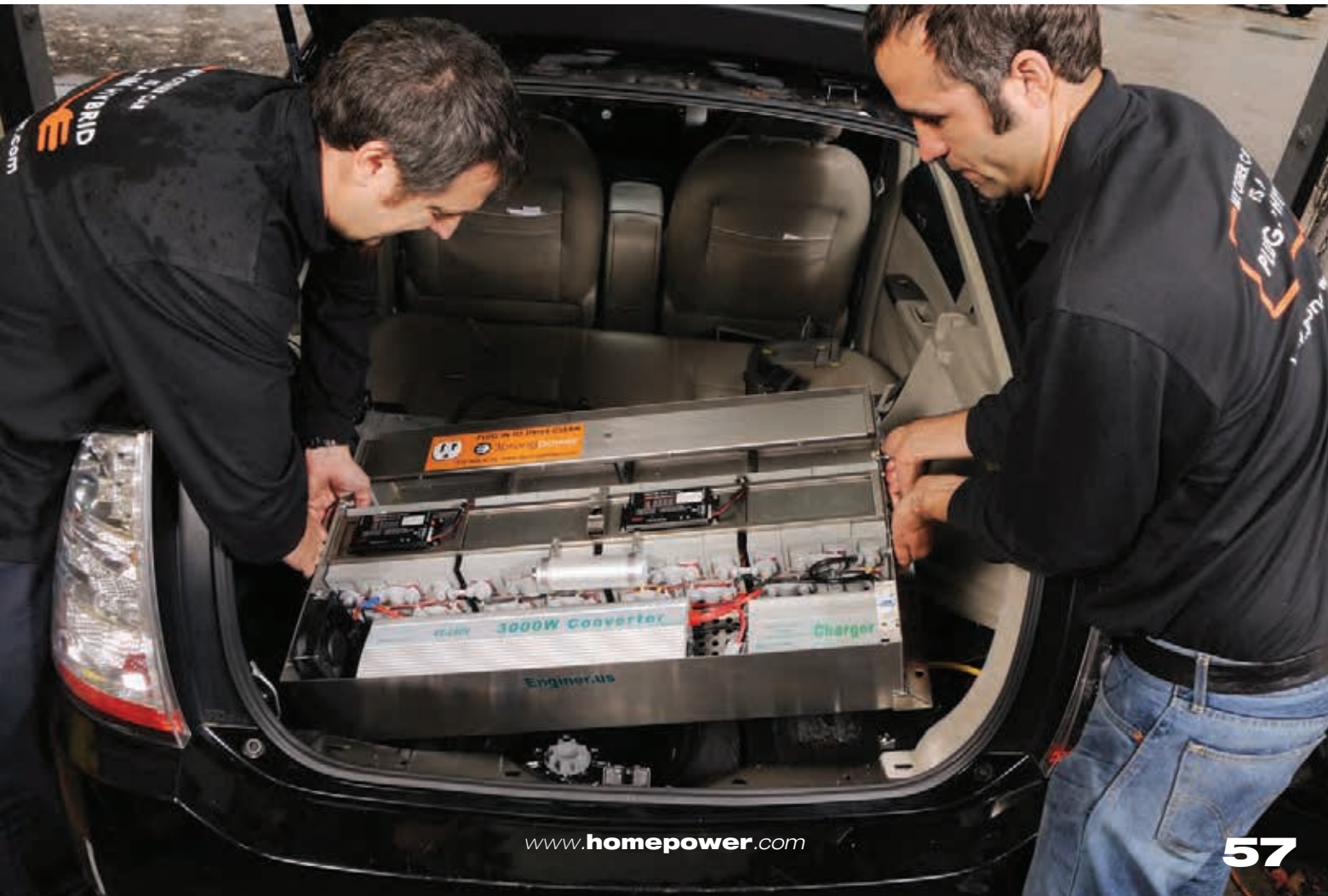
The new battery and charging module drops in above the spare tire.
