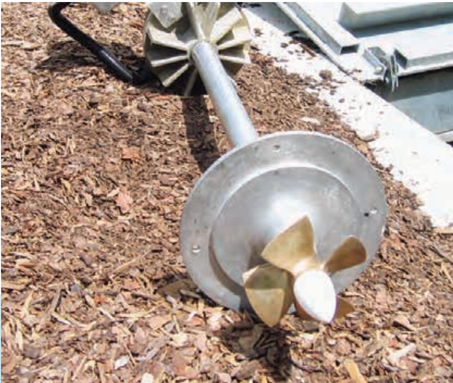
The ES&D turbine without its draft tube, showing the propeller.
