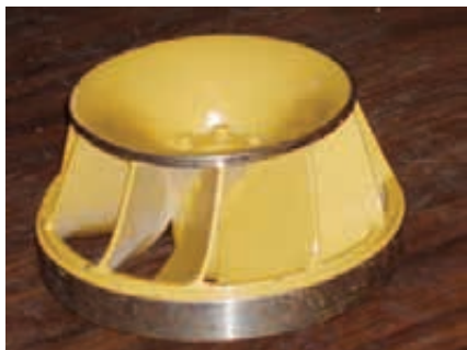
This Francis runner is an example of a reaction turbine, which is submerged in water and rotates with the force of water flowing through the equipment.
