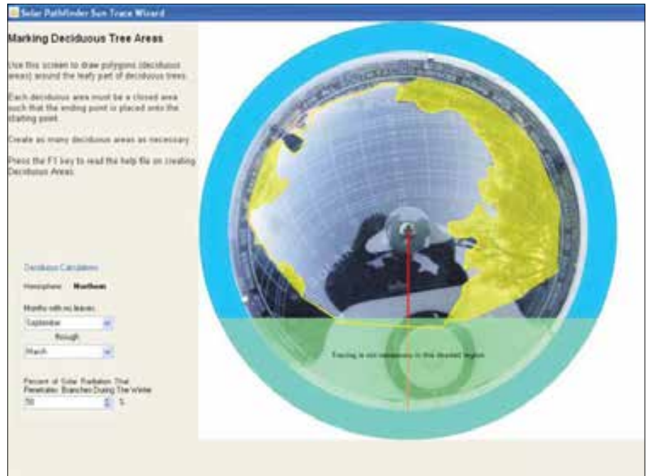
The Solar Pathfinder software calculated the usable solar irradiation at the site. The translucent yellow shading on the photo depicts deciduous trees.
