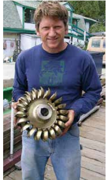
The author with the 10.5-inch Pelton runner for the Canyon Industries turbine.
