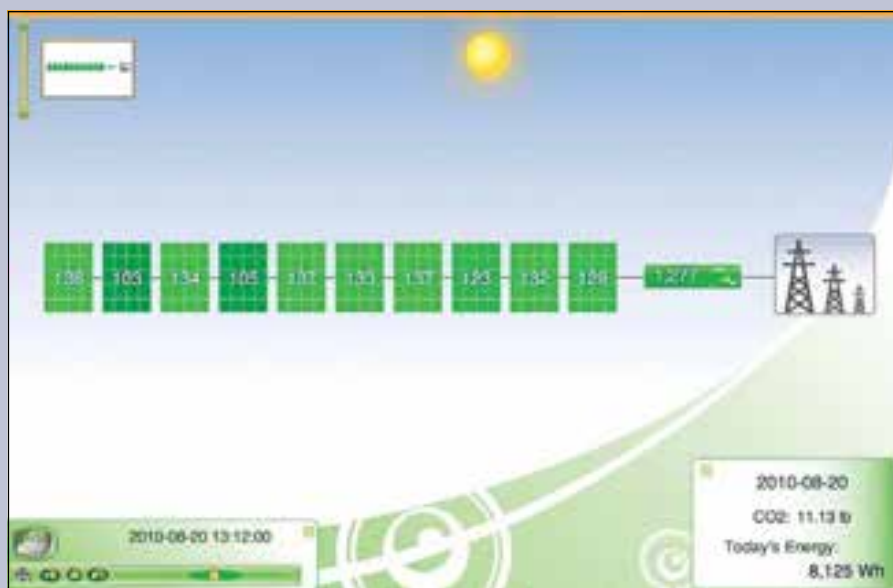
This screen shot shows lower wattages for modules No. 2 and No. 4. Module No. 8 is also slightly lower.
