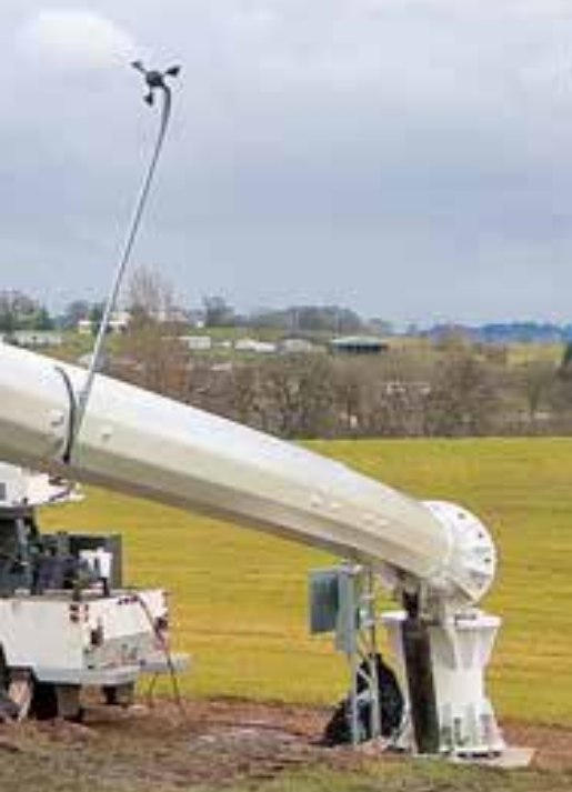
Tilt-up towers require a large, open site to raise and lower the tower, but guyed towers can be sited on cluttered sites and even between buildings.
