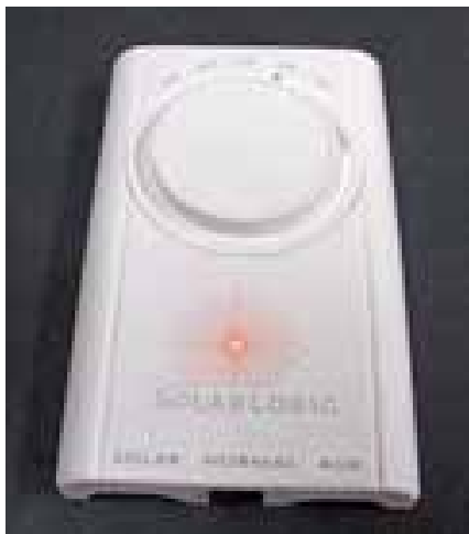
Two-stage thermostats allow custom tuning of the zones to optimize the solar versus boiler heat balance.
