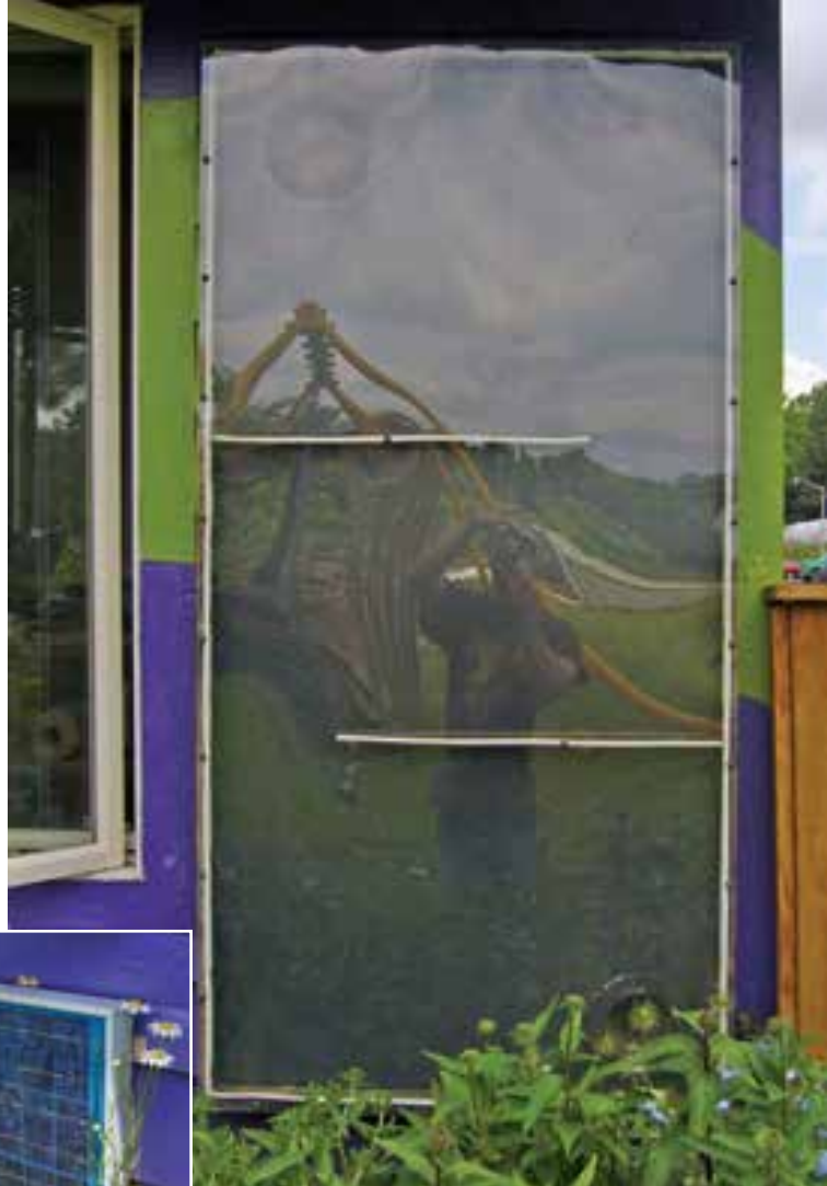
Above: The homemade 3- by 6-foot hot air collector augments space heating.
