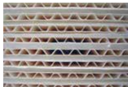
A closeup of the air-to-air heat exchanger core.
