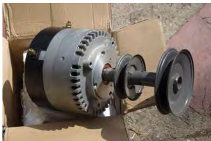
Above: The new Motenergy ME1004 with the stacked pulley in place.
