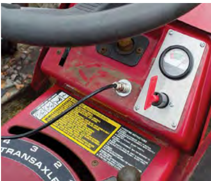
The voltmeter, power switch, and charger input receptacle—all conveniently mounted on the dashboard.
