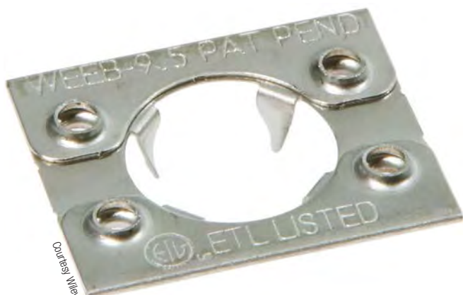
This WEEB grounding washer can be sandwiched between a module and its mounting rail. The protrusions bite into both, creating an approved ground path between them.
