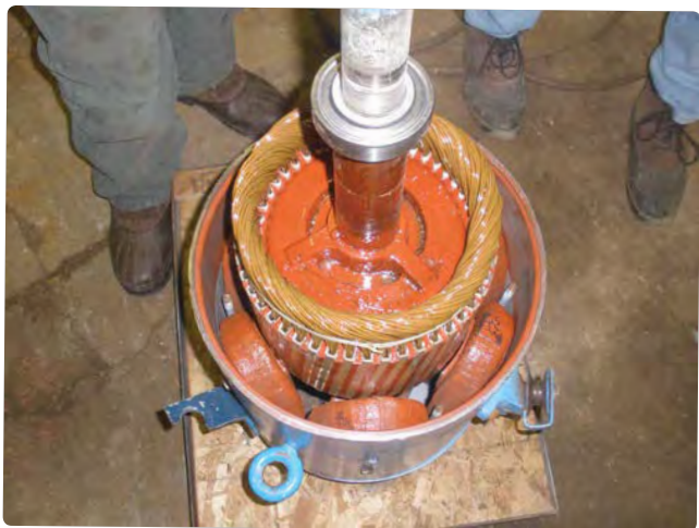
The front end of the generator. The blades would be attached to the long shaft.
