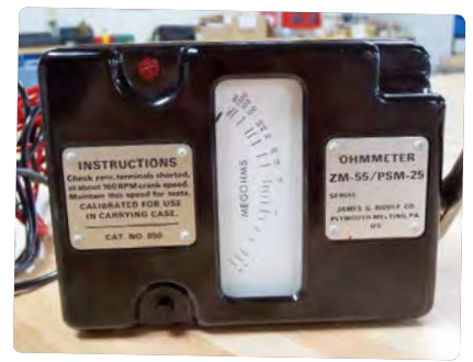
A megaohmmeter (megger) was used to test the THWN conductor insulation.
