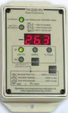
TriMetric TM-2025-RV includes enclosure
