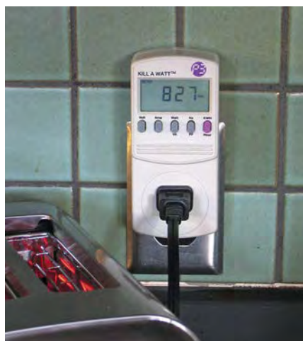
An energy meter like the Kill A Watt can help you measure common household 120 VAC loads.
