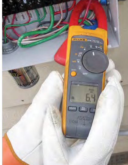
A clamp-on meter is used to measure the current while the array is connected to the inverter.
