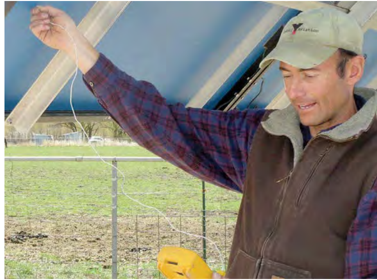
Placed against the back of a module, a sensor (attached to a meter) can be used to measure cell temperature. Be sure to take readings on several spots and average the results.
