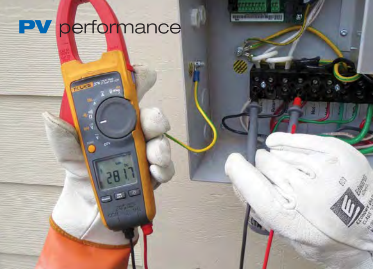
Measuring the array's operating voltage at the positive and negative terminals, with the array connected to the inverter.
