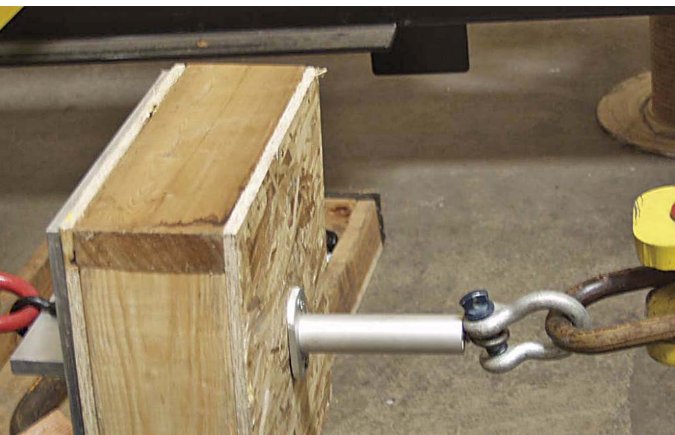
The sample section of SIP, with the solar rack standoff mounted and ready to be tested for pull-through strength.
