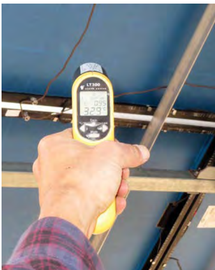
A temperature gun checks infrared radiation to give quick readings of cell temperature.
