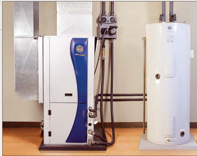
Typical forced-air, ground-source heat pump equipment. In this case, the system includes a desuperheater to provide domestic hot water, which is stored in the tank on the right.
