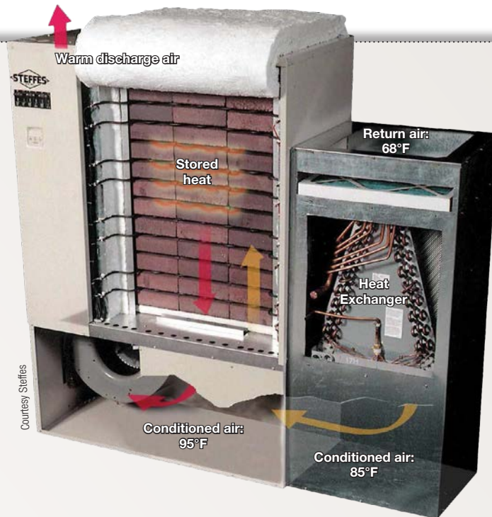
An electric thermal storage unit. Note that the side insulation has been rolled back to reveal the ceramic bricks inside the unit.
