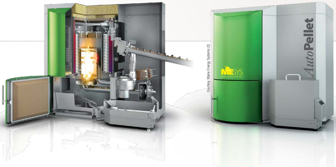
This automatic pellet boiler manufactured by Maine Energy Systems includes an auger that moves pellets from a nearby storage bin to a self-cleaning combustion chamber.
