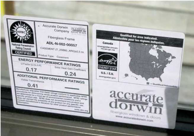
NFRC window labels include U-factor, solar gain, transmittance, and optionally, air leakage and condensation resistance.
