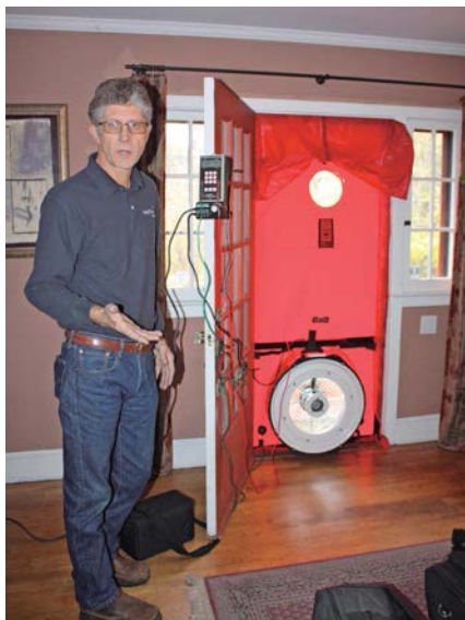
A blower-door test determines the amount of air infiltration a home has, expressed in air changes per hour (ACH).
