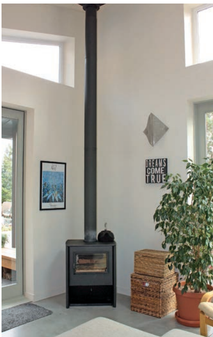
The small Avalon Camano wood heater provides enough heat from one firing to keep the superinsulated home warm for up to five days.
