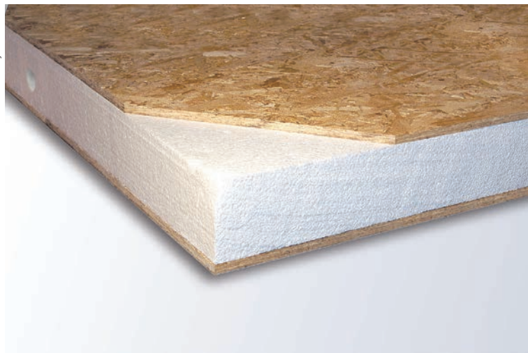
Structural insulated panels (SIPs) are one of the best-insulating wall systems, providing good R-value, limiting air infiltration, and minimizing thermal bridging.
